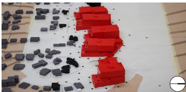
Image 2B: Wind Tunnel Study Model – Proposed Configuration
