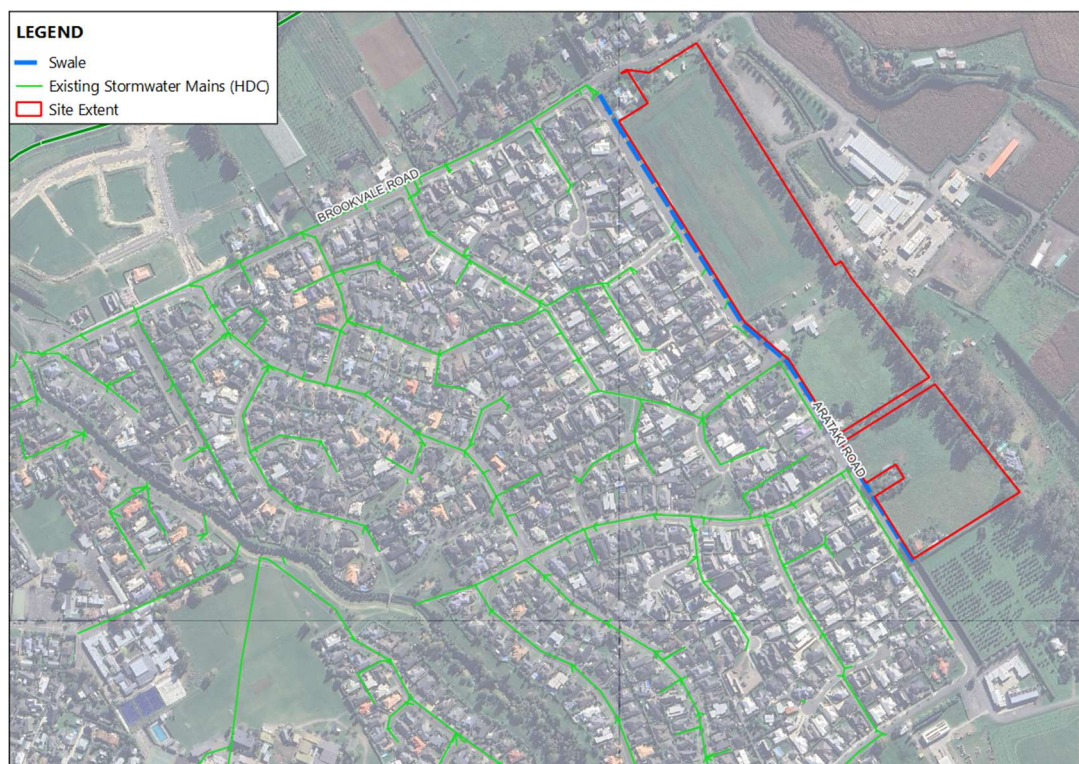
Figure 4: Existing stormwater network (Source: HDC online maps)
