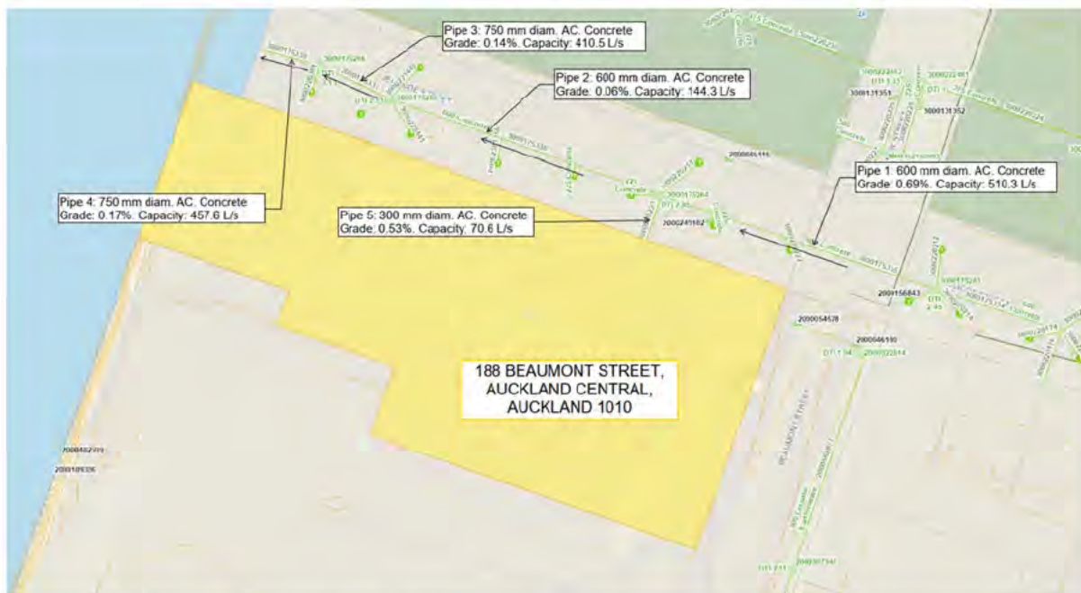
Figure 2-2: Existing stormwater network within proximity to site (sourced from Auckland Council GeoMaps)
