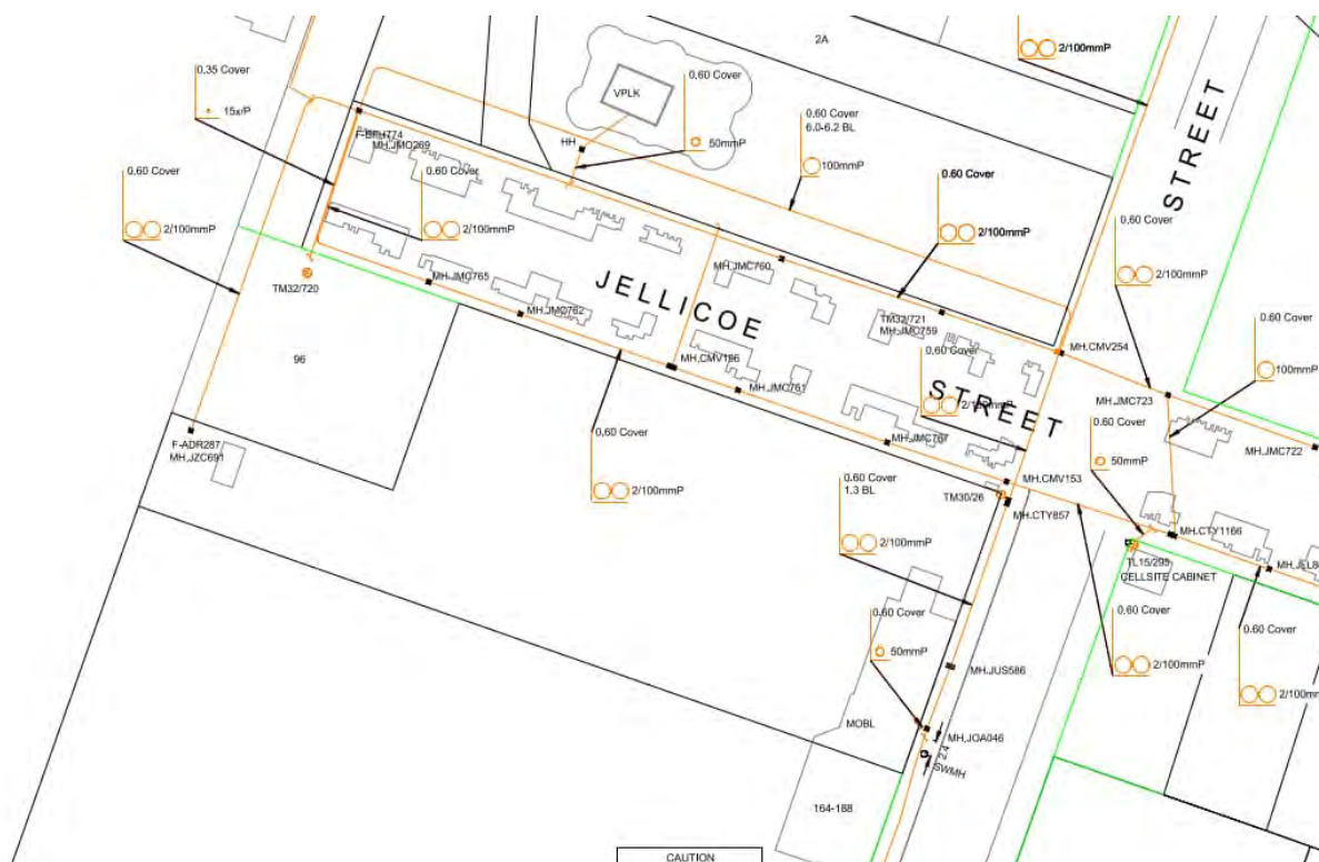
Figure 5-3: Chorus fibre network (network in orange, property boundaries in green) (sourced from BeforeUDig response)
