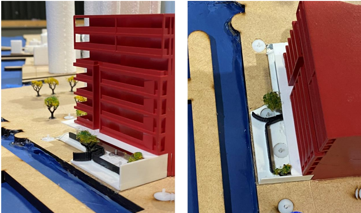
Figure A-10. Curved solid screen added on the western side of the proposed building, in addition to the final mitigation measures described in Section 9.
