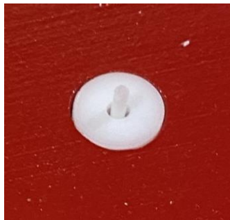
Figure 15. Close up photo of the surface level wind speed sensor (i.e. Irwin probe).
