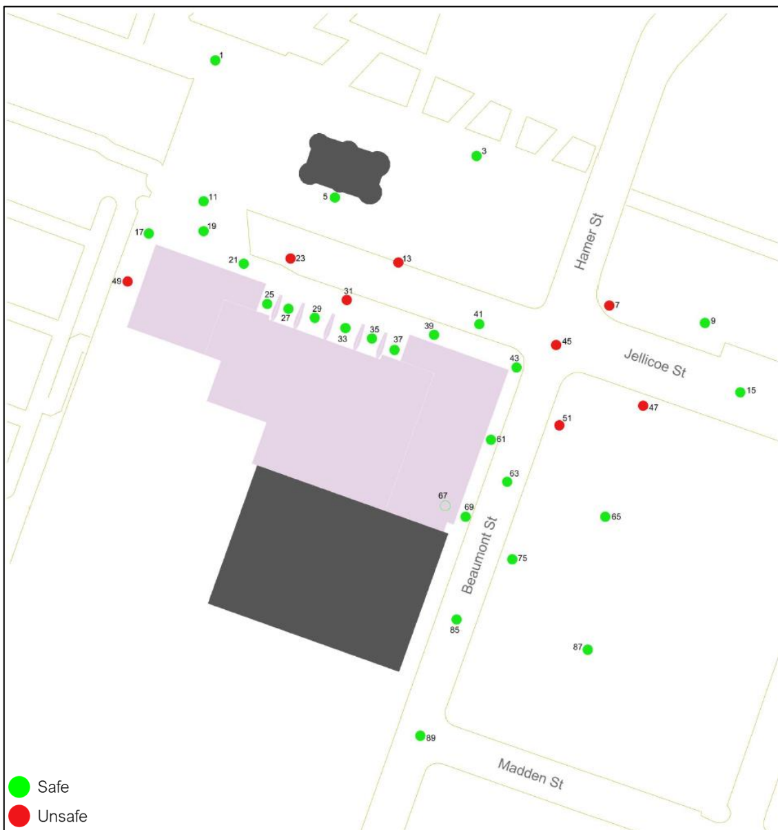
Figure 22. Pedestrian wind safety conditions of the proposed configuration , assessed against criteria in the AUP OIP.
