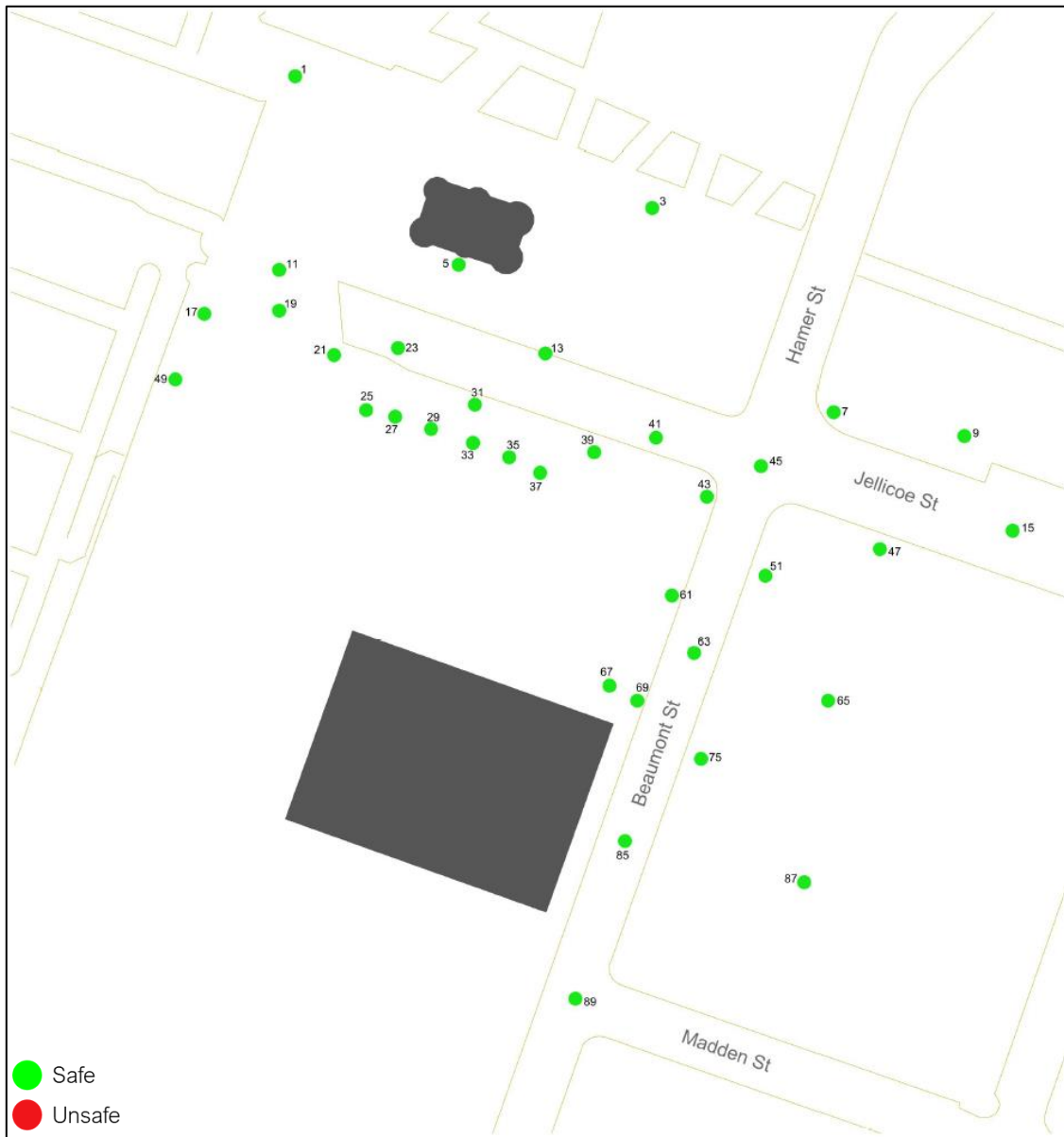
Figure 20. Pedestrian wind safety conditions of the existing configuration , assessed against criteria in the AUP OIP.
