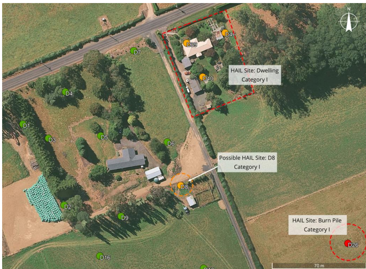
Figure 21: Sampling locations across the northern end of the site. Locations denoted in red indicate samples with contaminant concentrations that exceed the Commercial/Industrial SCS/SGV, and locations coloured orange indicate samples with contaminant concentrations above background but below the Commercial/Industrial SCS/SGV. Locations coloured green indicate samples consistent with predicted background. Areas outlined in red indicate identified HAIL sites, and areas outlined in orange indicate possible HAIL sites (aerial imagery sourced from Google Earth, imagery © 2025 Airbus).
