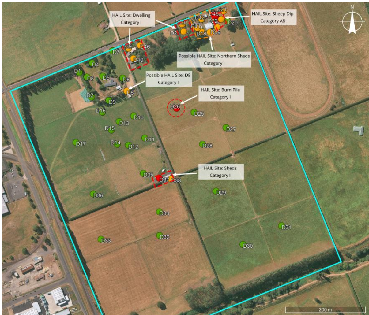
Figure 19: Sampling locations across the site. Locations denoted in red indicate samples with contaminant concentrations that exceed the Commercial/Industrial SCS/SGV, and locations coloured orange indicate samples with contaminant concentrations above background but below the Commercial/Industrial SCS/SGV. Locations coloured green indicate samples consistent with predicted background. Areas outlined in red indicate identified HAIL sites and areas outlined in orange indicate possible HAIL sites (aerial imagery sourced from Google Earth, imagery © 2025 Airbus).
