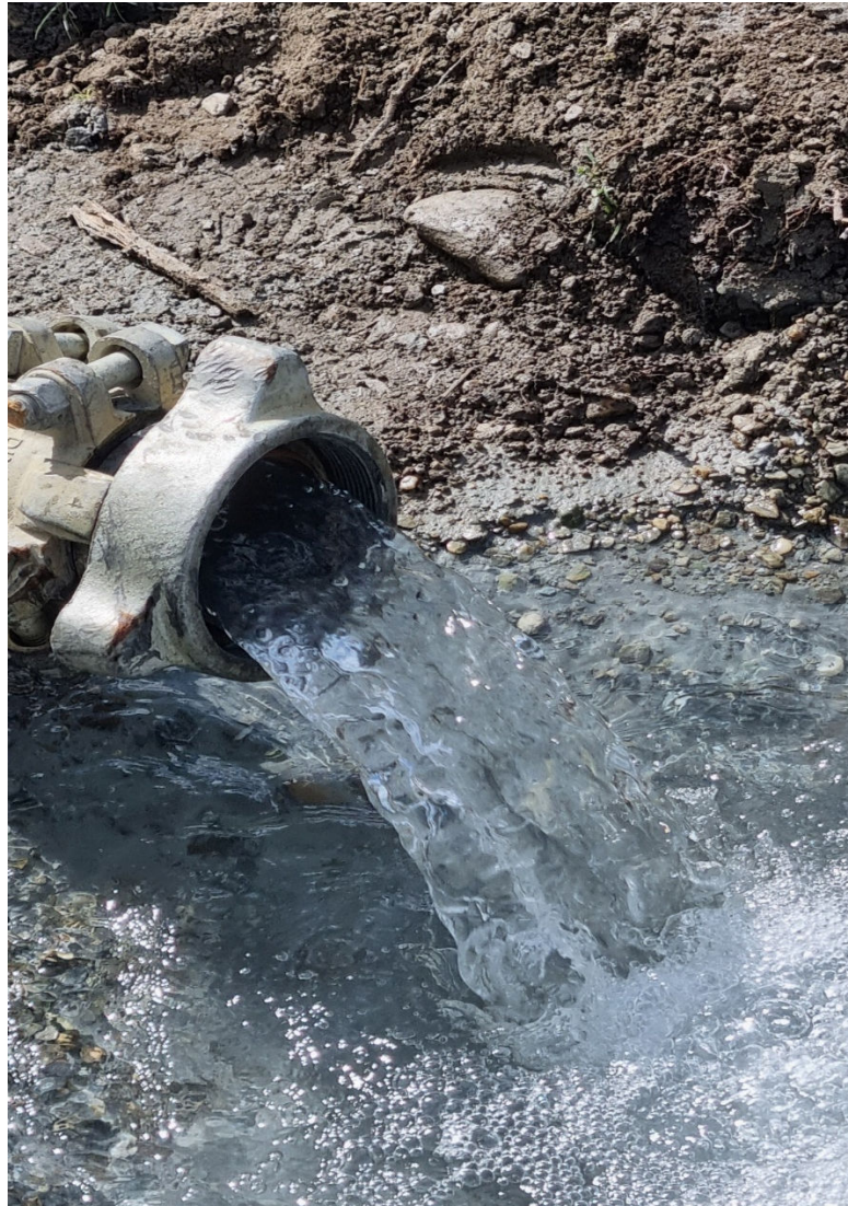
Photograph 2 Much clear and lower turbidity water near end of constant rate test in 140
