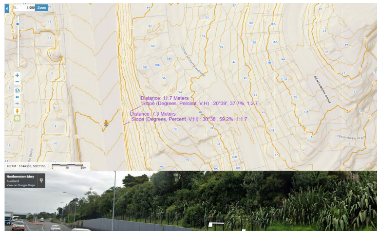
Figure 1: General example of contours reflecting motorway cutting works. Note, this example is on the opposite side of the motorway than the busway alignment.
