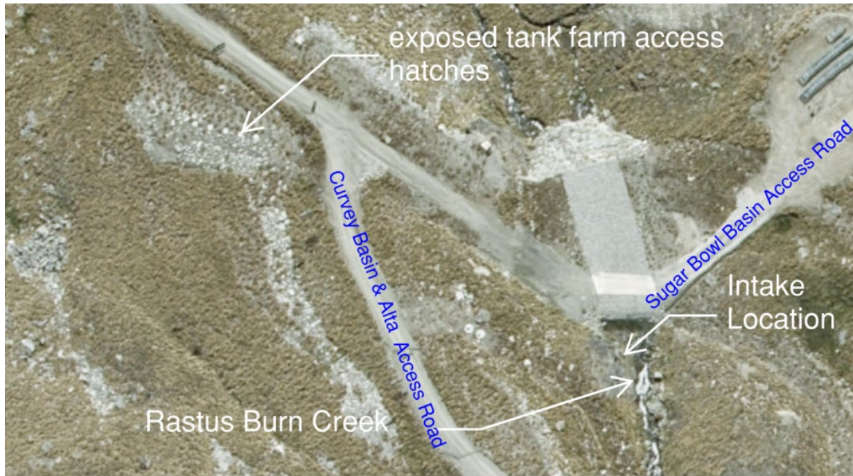
Figure 3. Location of potable water intake in the Rastus Burn and tank farm lids
