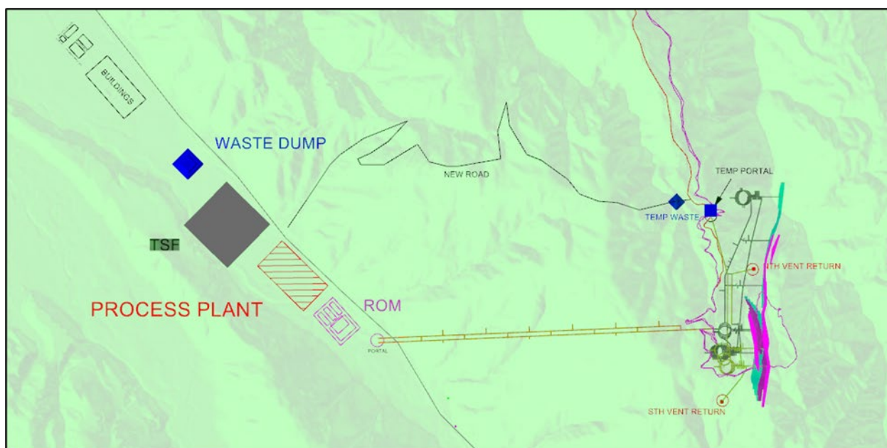
Figure 17-3 New (temporary) haul road
