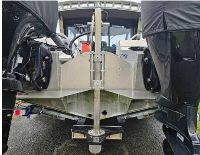
Figure 4: MBES Sonar stern mounted strut in deployed position.
