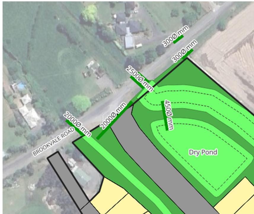
Figure 11 Proposed Brookvale Road Culverts
