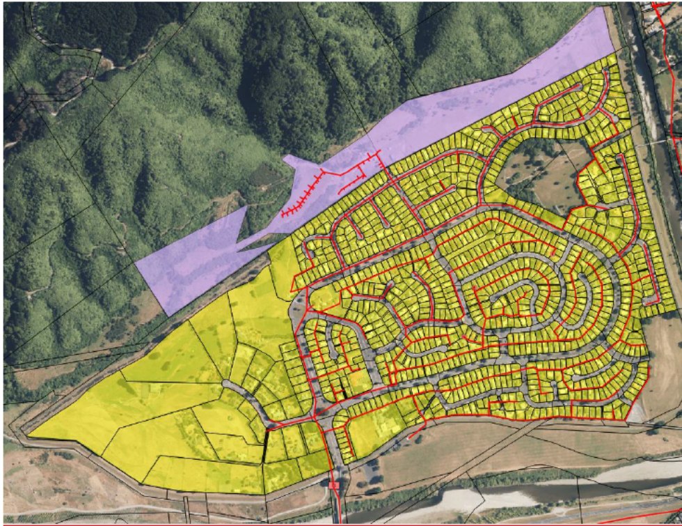
Figure 38 - Totara Park WWPS catchment, as existing
