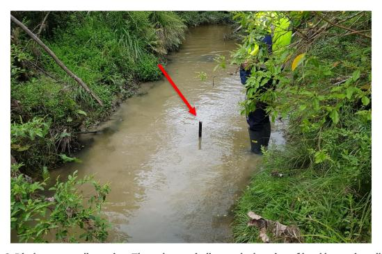
Photo 2. Discharge sampling point. The red arrow indicates the location of level logger installation.
