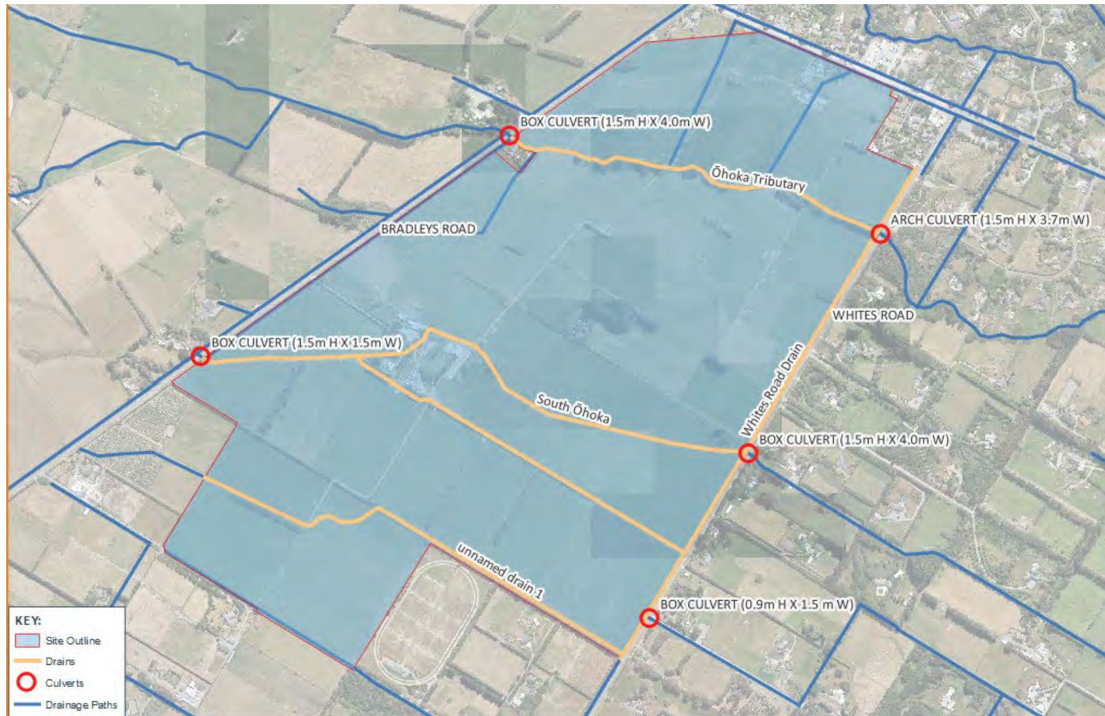
Figure 2: Existing Stormwater infrastructure.
