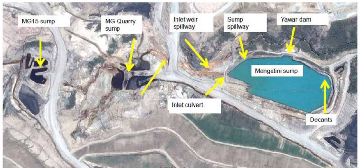
Figure 4 Mangatini Sump Treatment System
