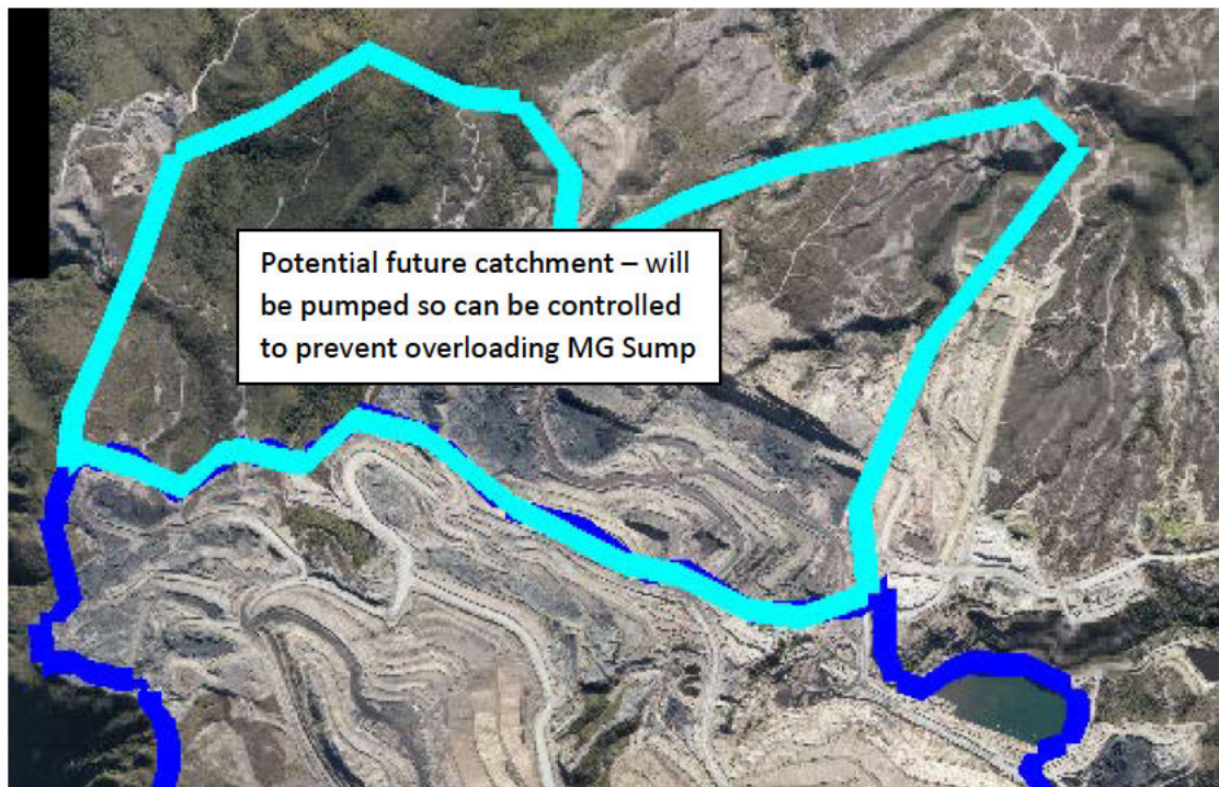
Figure 5: Planned Future area to be treated using the Mangatini Sump
