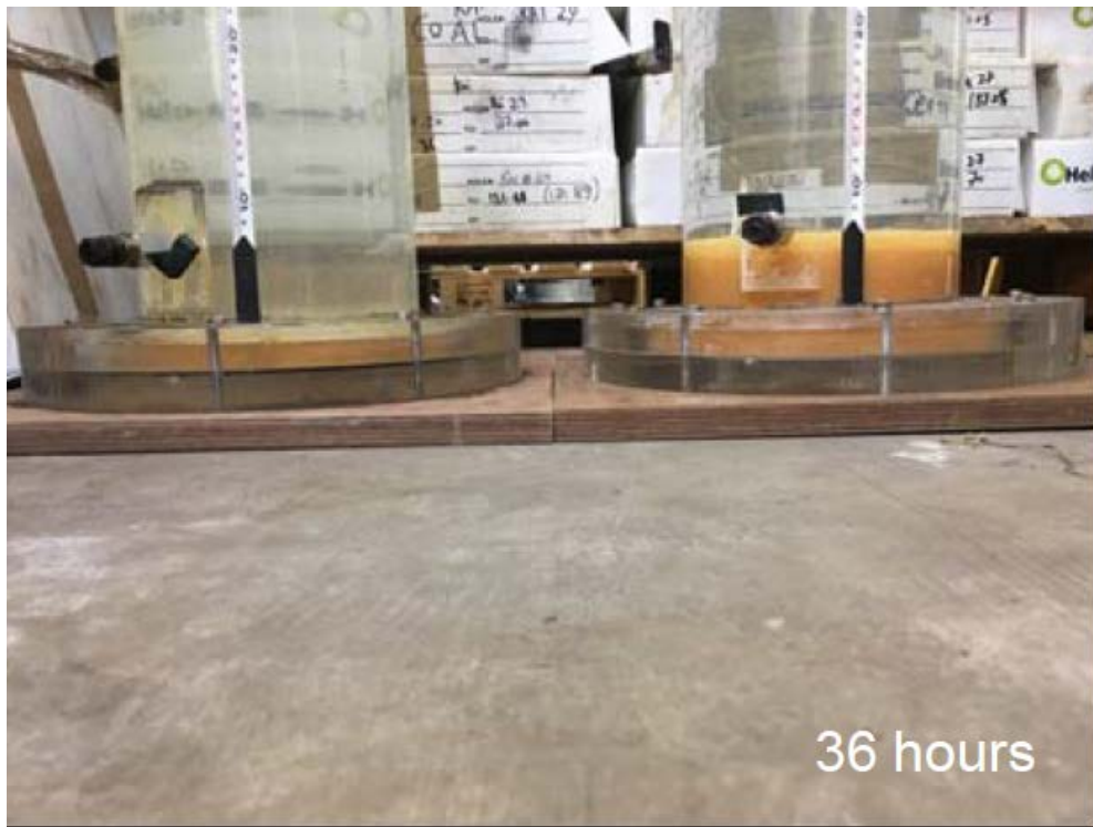
Figure shows site AMD treated with UFL to the left and with CaO to the right
