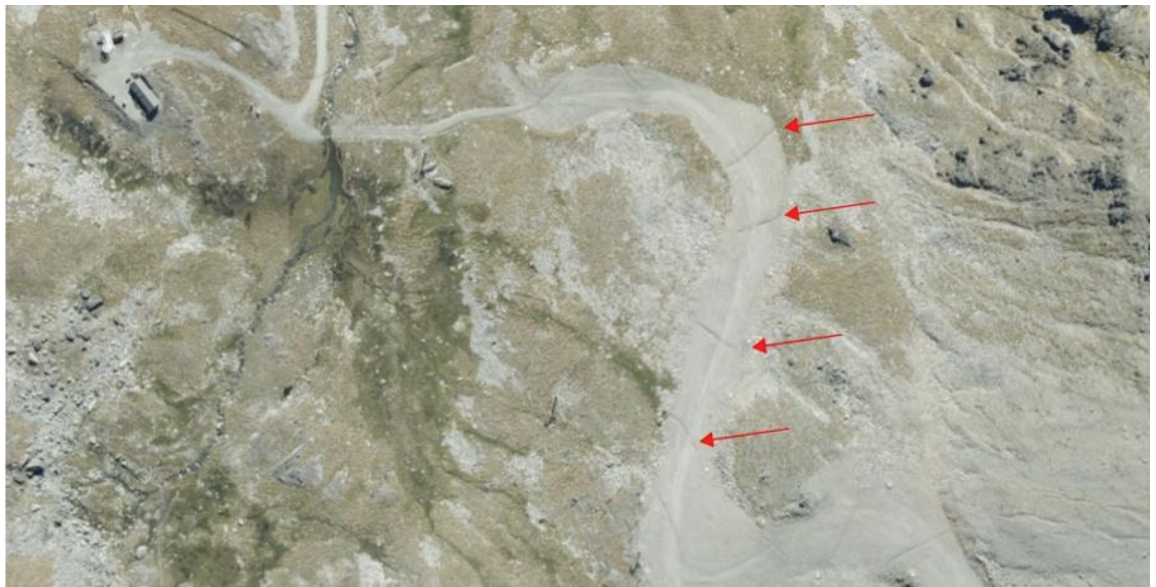
Figure 3-23: Stormwater channels to maintain surface sheet flow as much as possible, as used in the Rastus Burn catchment (Stantec, 2026d).
