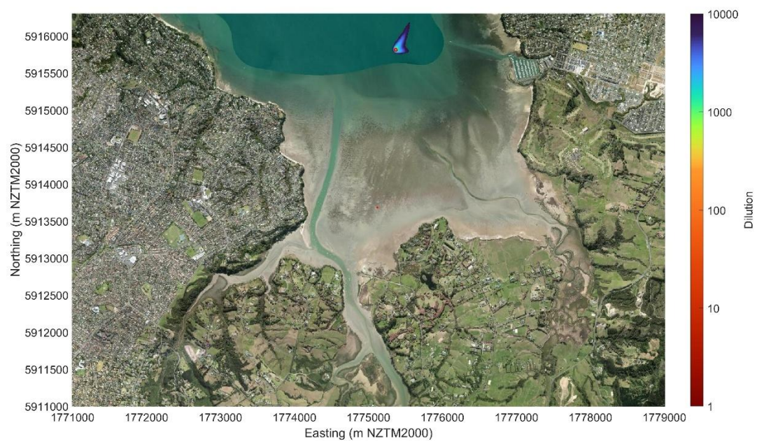
Figure Appendix D.9: 50 th percentile dilution factor map with 1000-fold dilution contour shown in red. Dilutions less than those shown occur 50% of the time.
