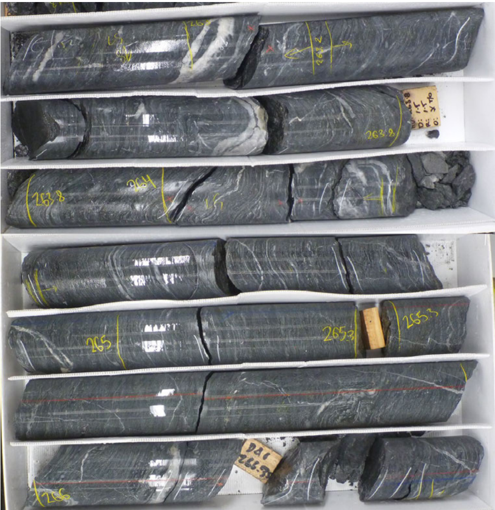
Inset 7: Core photo example from ddh7837 of rock mass conditions within a modelled stacked ore lode.
