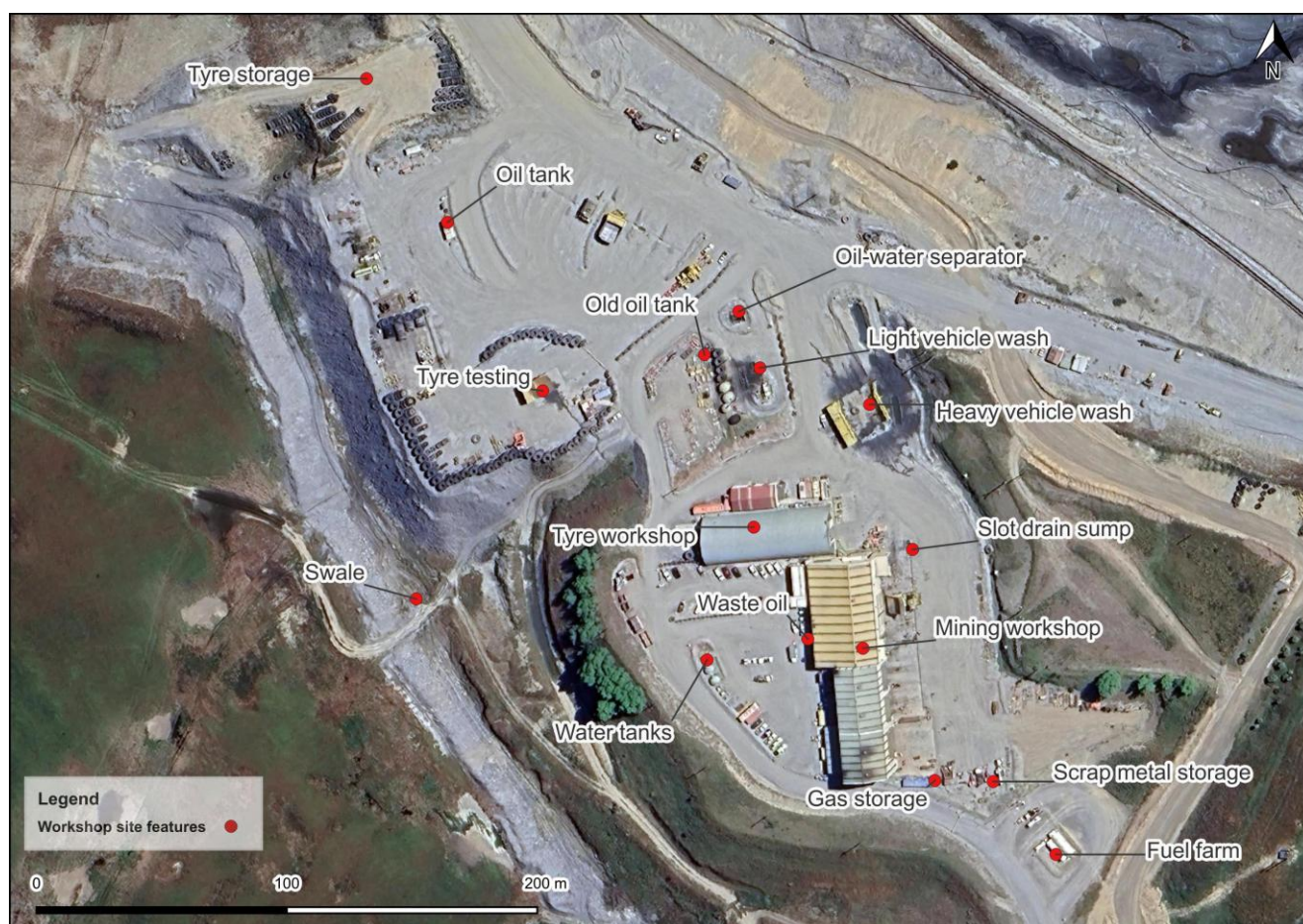
Figure 3. Key features in Workshop area
