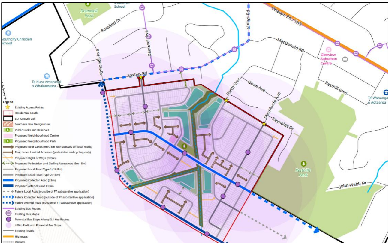
Figure 36: Residential Development – Road Carriageway Width Hierarchy
