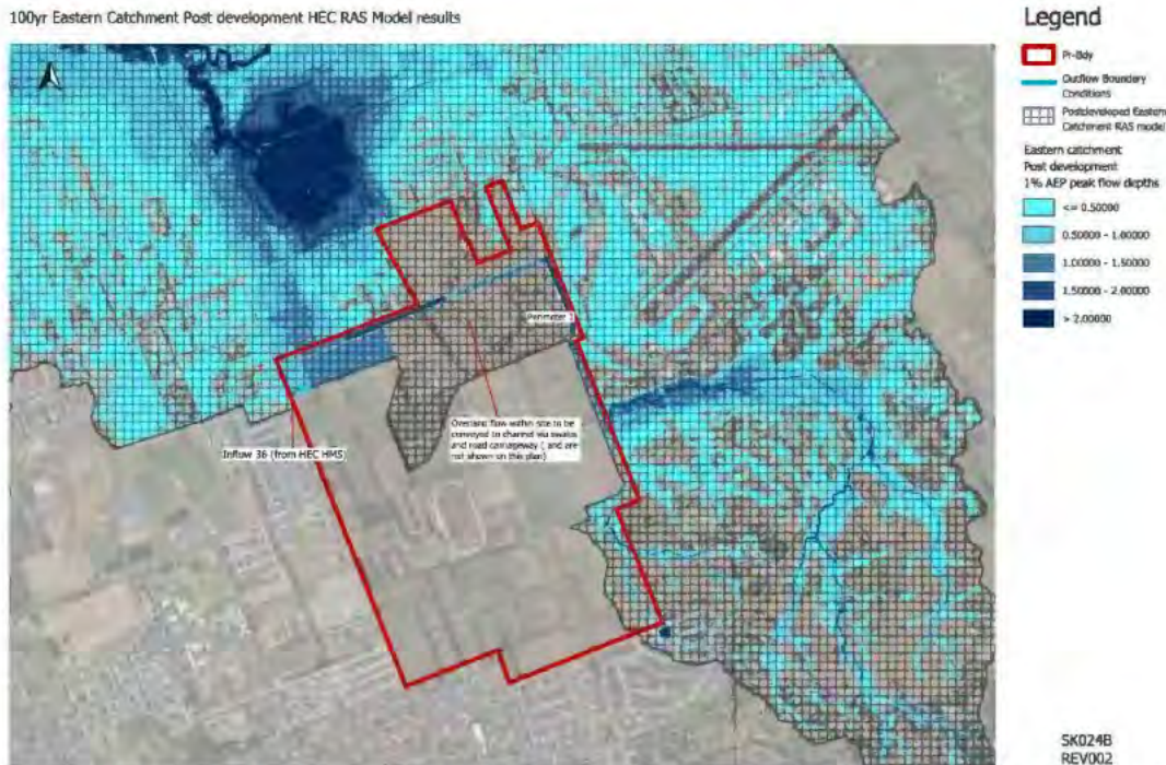
Figure 15: Extent of flooding within Perimeter Swale and Proposed Pond 1 for the diversion of upstream catchment in Eastern Catchment
