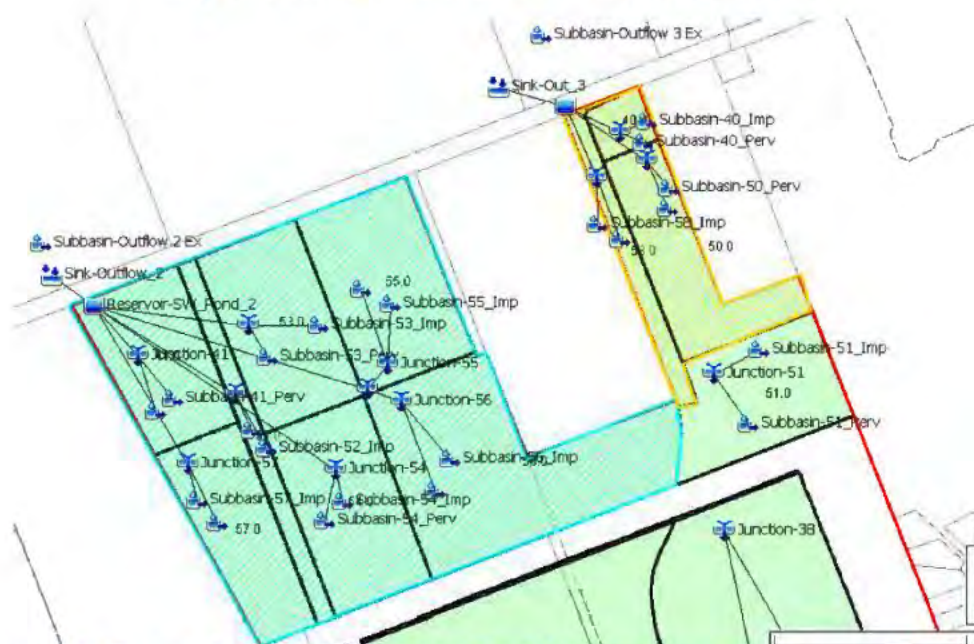
Figure 4.4 –Eastern Catchment 1%AEP HEC-HMS Model Set-Up for Stormwater Pond 2&3
