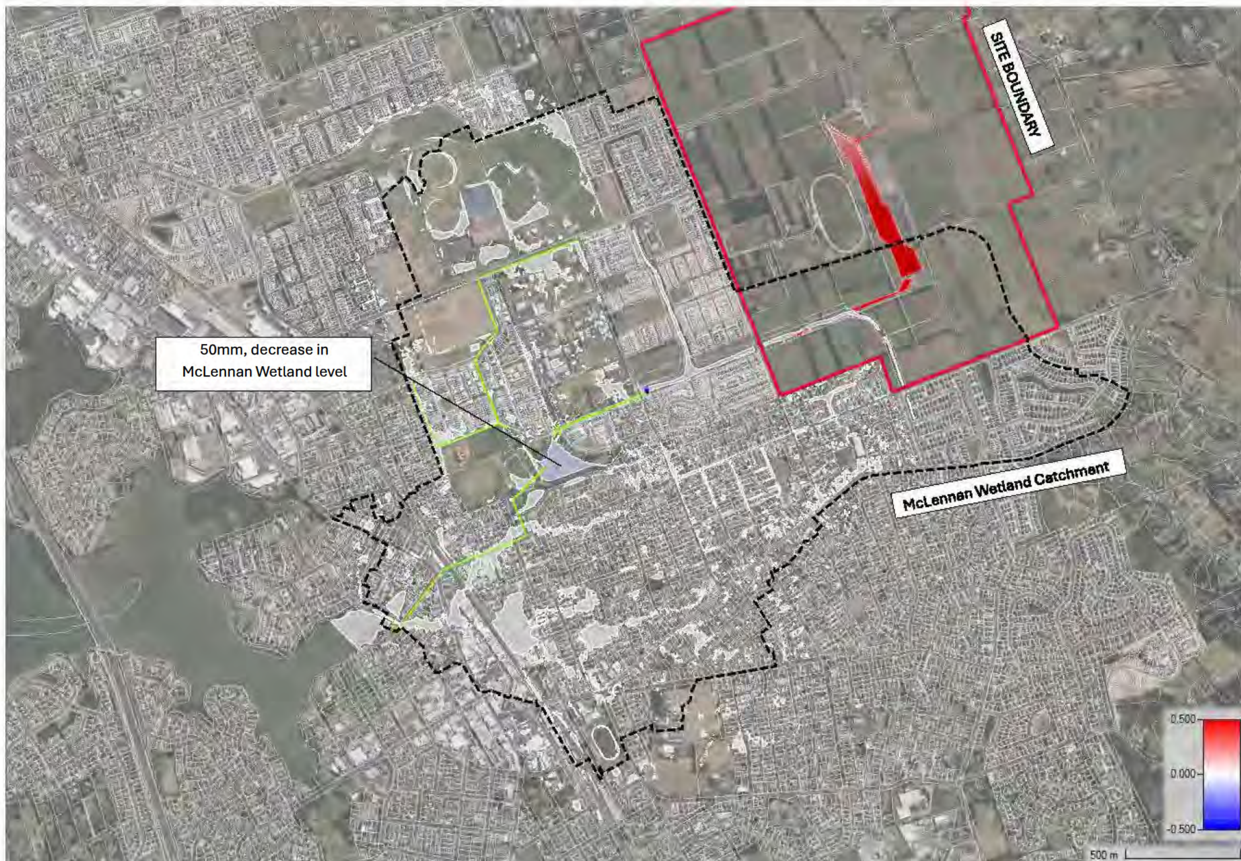
Western Catchment 50%AEP – Flooding level Comparison Extents (Post Development minus Existing: ie blue = decrease and red = increase)
