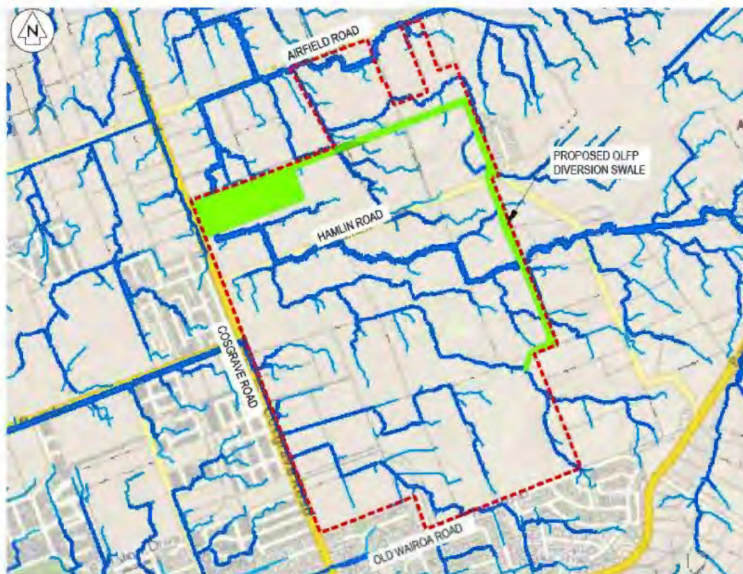
Figure 14: Perimeter overland Flowpath Diversion Swale
