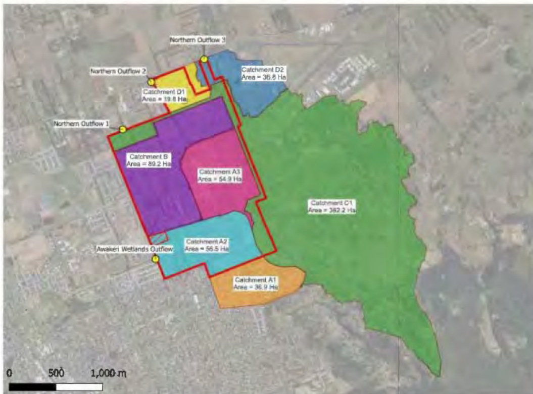
Figure 9: Post – Development Stormwater Catchment Plan for 1% AEP storm event
