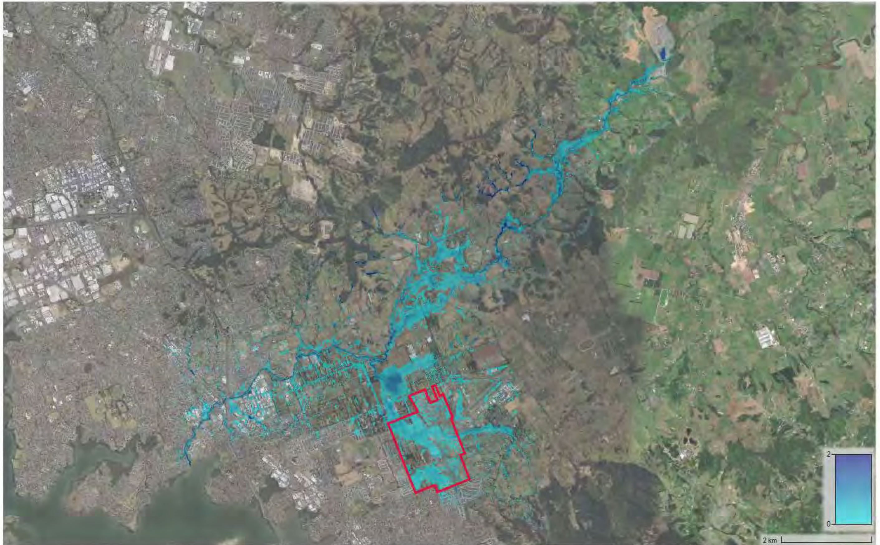
Eastern Catchment 50%AEP – Existing Flood Extents
