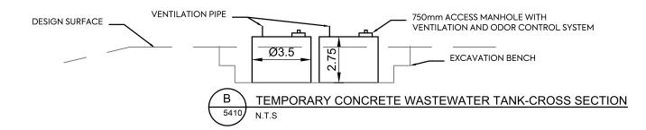
NOTE: TANK ANCHORING MAY BE REQUIRED IF GROUNDWATER TABLE IS HIGH.
