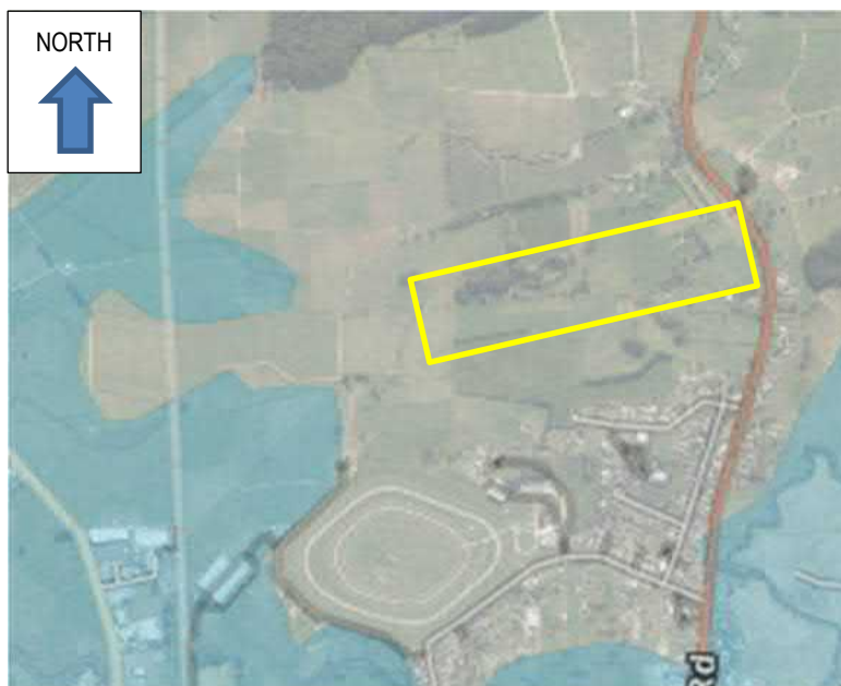
Figure 4.1: Extent of flooding with the development area during a 1 in 100-year flood.
