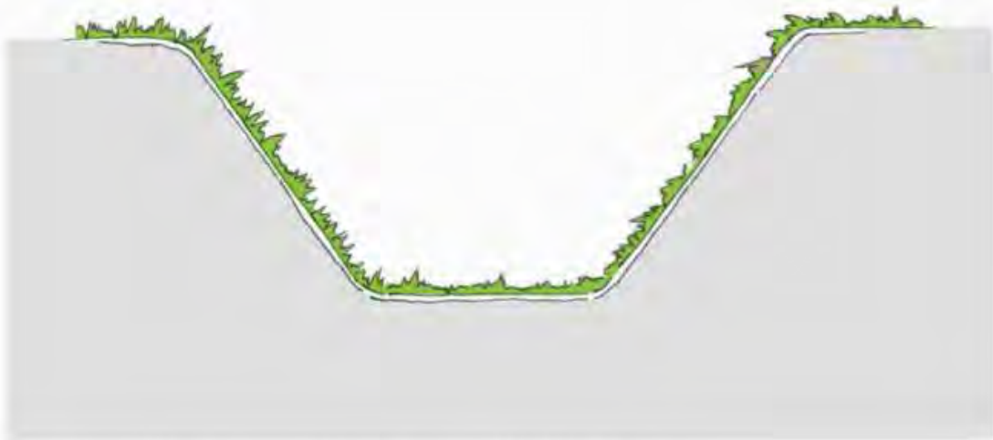
Grass-Lined Flow Channel for Low Flow and/or Flat Gradients
