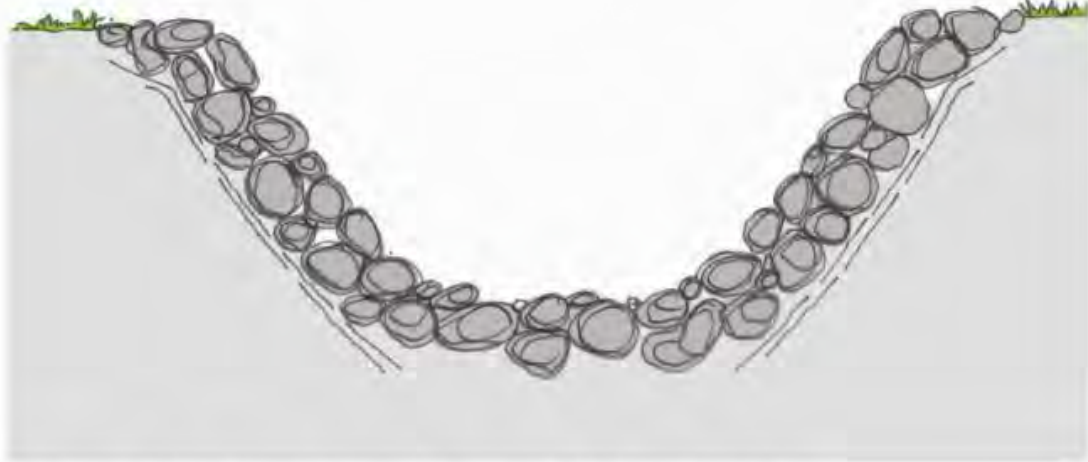
Rock-Lined Flow Channel for High Flow and/or Steep Gradients
