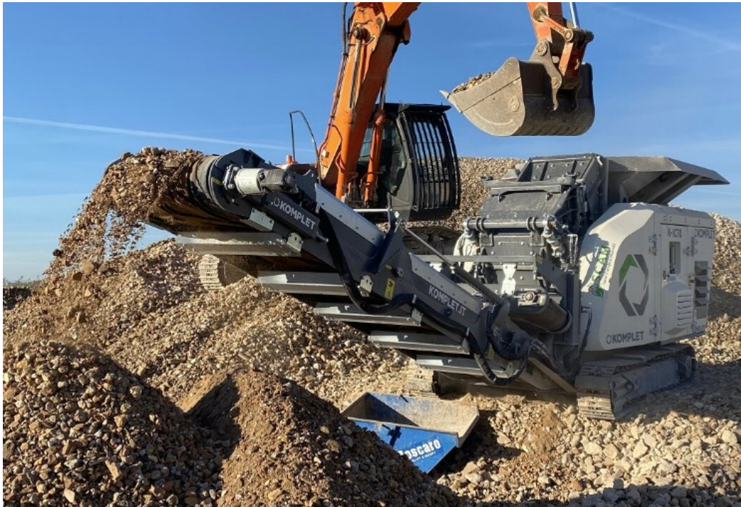
Figure 3-27: Typical Mobile Crushing and Screening Plant
