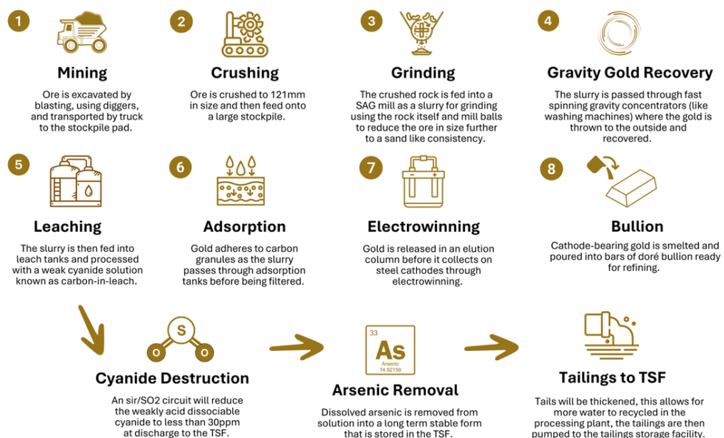
Figure 3-11: Proposed Ore Material Processing Stages
