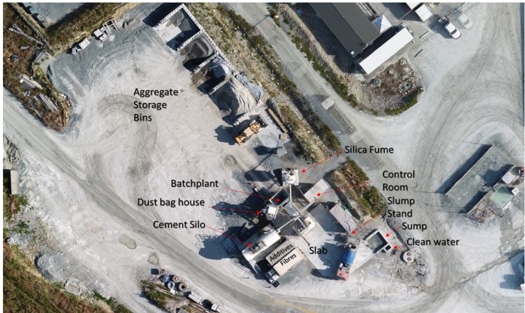
Figure 3-15: Example Concrete Batching Plant Layout
