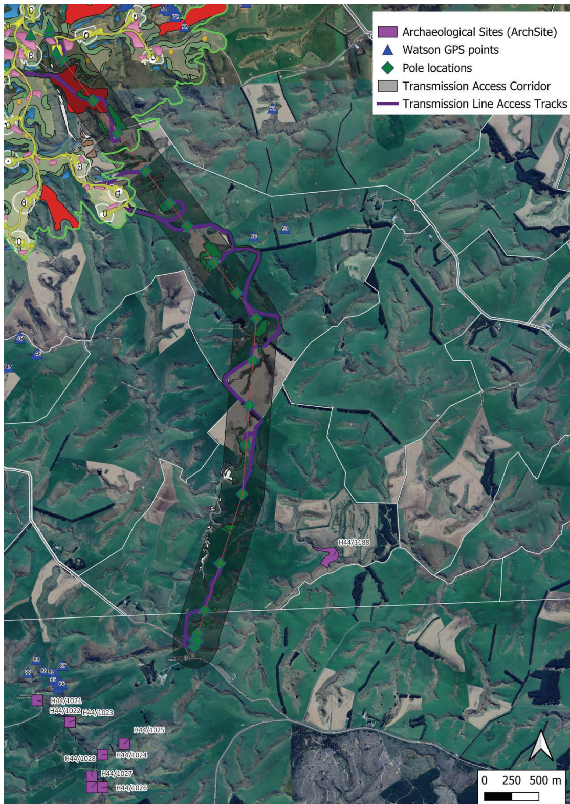
Figure 12. Proposed 110 kV transmission line from the wind farm to the National Grid via the 110 kV Halfway Bush – Roxburgh Line with proposed poles and access tracks. The locations of recorded archaeological sites are shown in the vicinity (NZAA H44# and Watson #)
