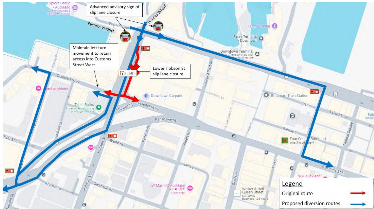
Figure 20: Lower Hobson Street slip lane diversion routes for Princes Wharf and Eastern Viaduct
