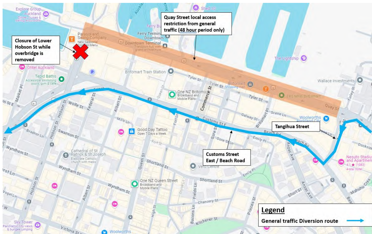
Figure 14: Lower Hobson Street pedestrian overbridge removal: Quay Street proposed local access restriction
