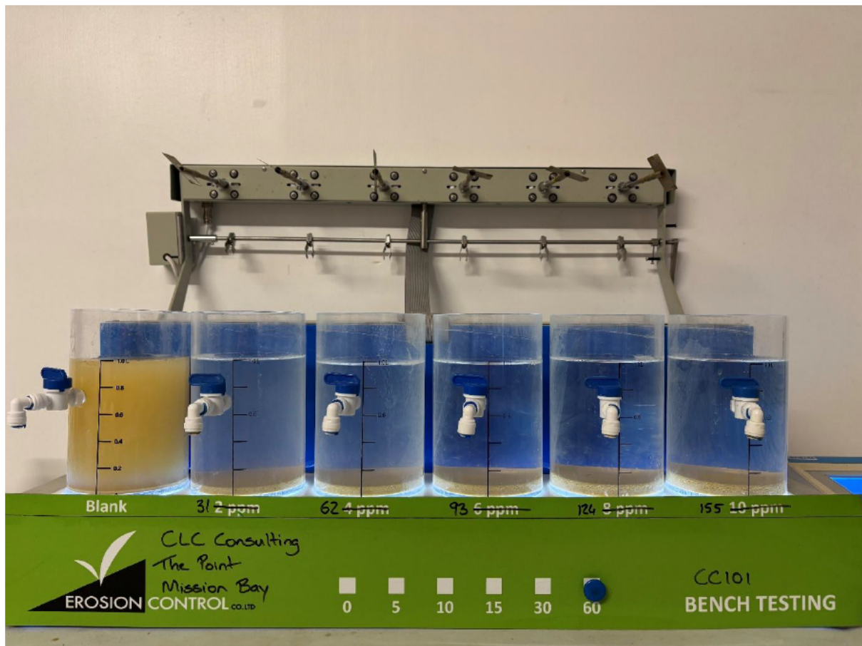
CATCHMENT SAMPLE: Chemiclear 101 on the Soil Sample after 60 minutes settling.
