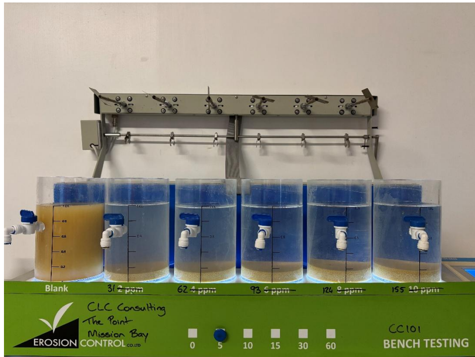
CATCHMENT SAMPLE: Test Results of Chemiclear 101 after 5 minutes settling
