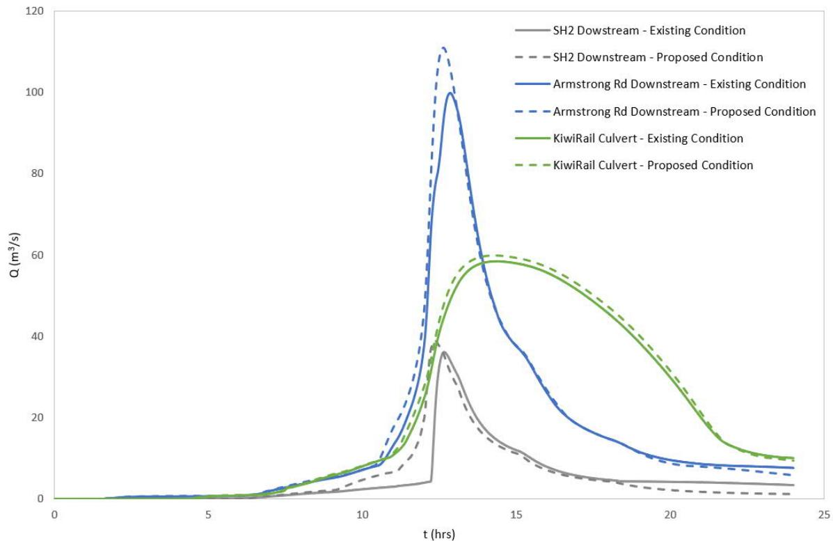
Designer response: At the roads, the upsizing of the existing culverts results in a 0.15m increase in the peak flow depths during large storms which does not significantly alter the existing high risk due to the overtopping. The impact of the upsized culverts on the risks due to road overtopping were not a major concern to the Regional Council.
