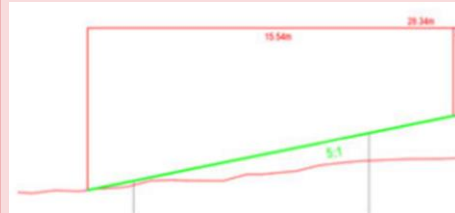
Figure 48: Engineering cross-section of diversion channel/bund
