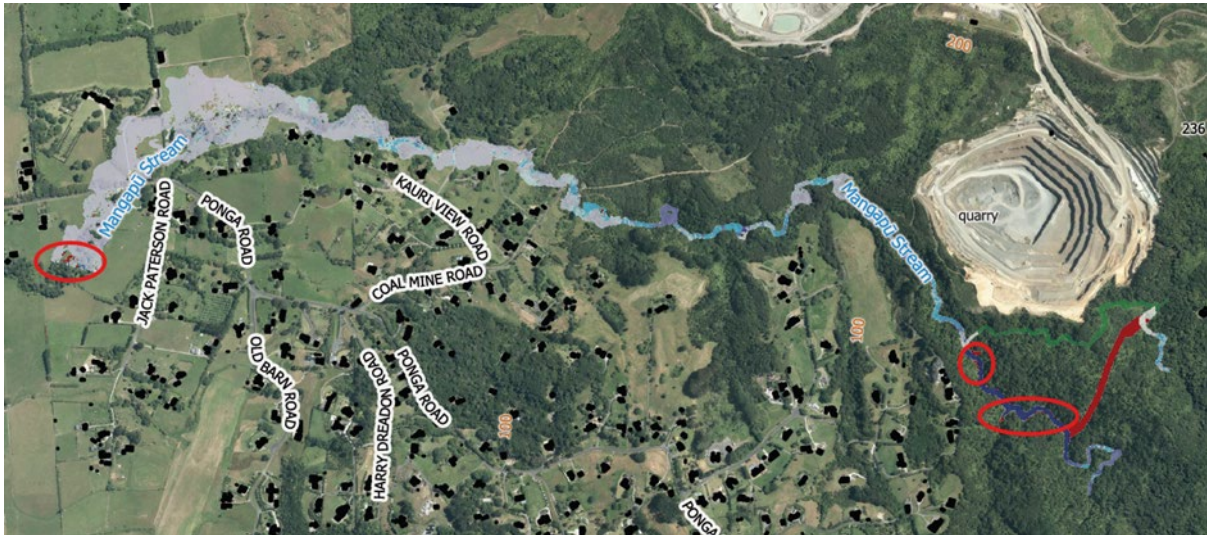
Figure 13: Red circles highlighting areas where flooding will occur post-development that did not pre-development
