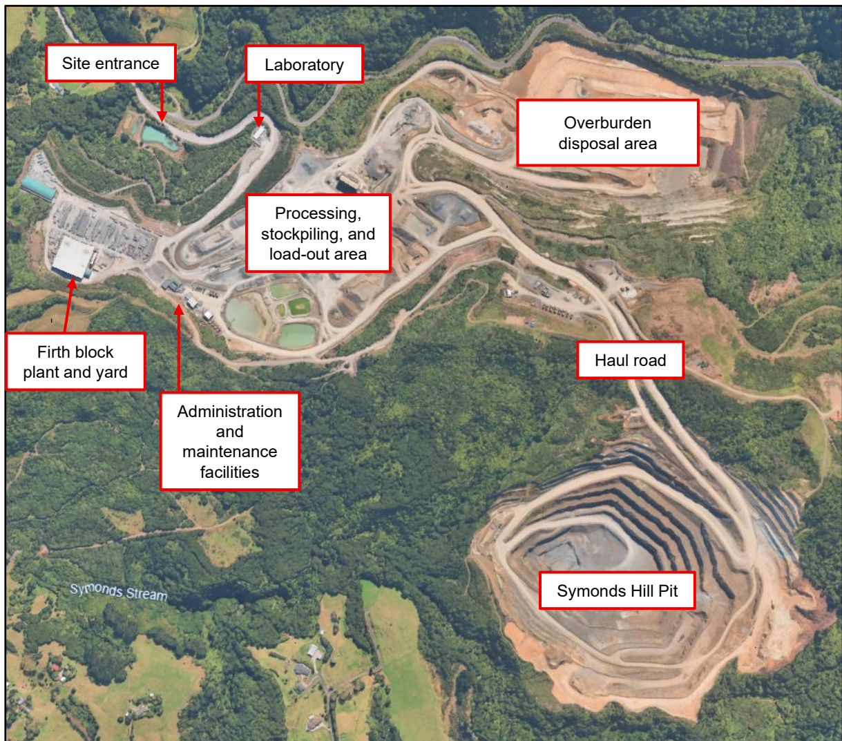
Figure 2: Existing layout of Hunua Quarry
