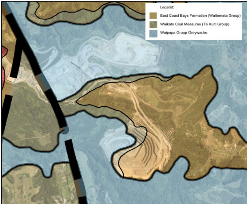
Figure 7: Geological map for the Hunua Quarry. Bold dashed lines indicate the location of the Drury Fault system. (Source: Appendix B12.4.8 Hunua Quarry Geotechnical Assessment, prepared by Tonkin & Taylor)
