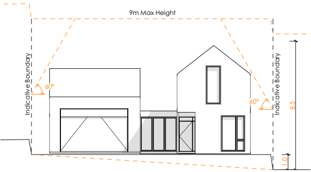
Street Elevation cross fall site
