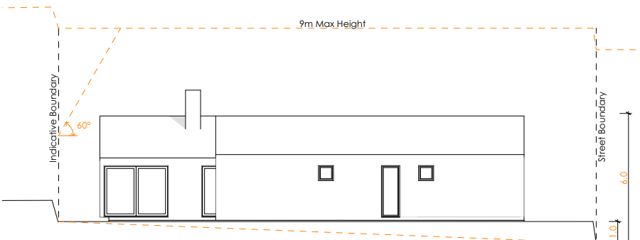
Side Elevation cross fall site
