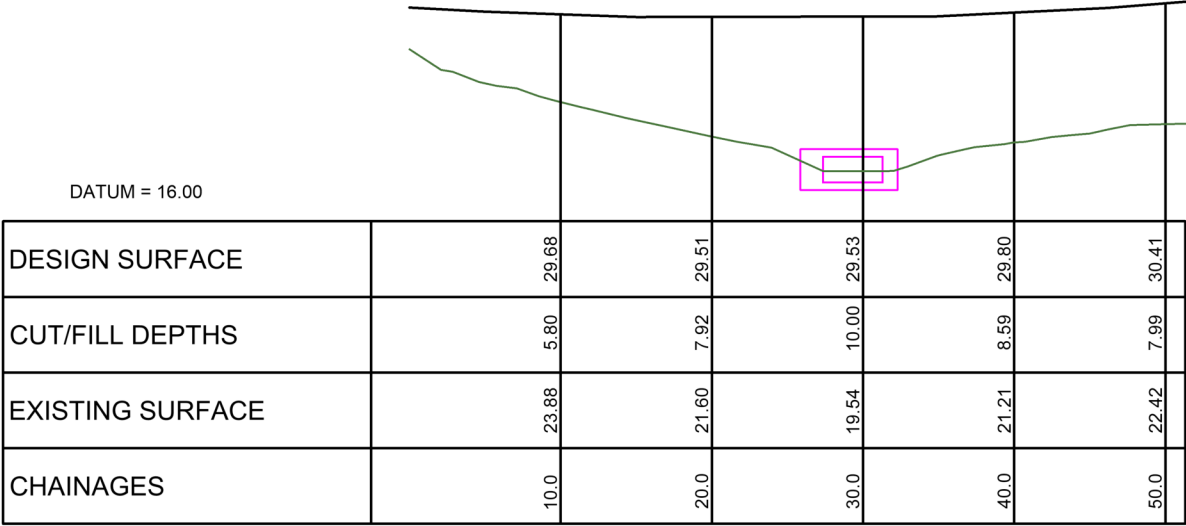
Culvert 11 - ELEVATION VIEW
