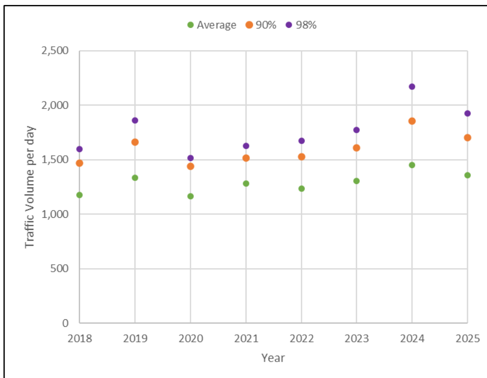
Figure 3-1: Annual traffic volumes on SH7 South of Inangahua River
