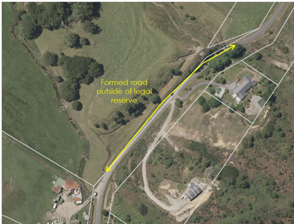
Figure 7-1: Formed road outside legal road reserve
