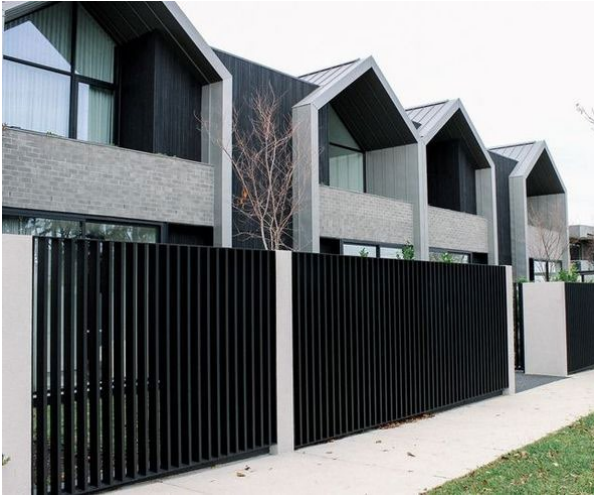
1.4 -1.8M HEIGHT SLATTED FENCE USE: JOAL AND STREET FACING BOUNDARIES WHERE GREATER PRIVACY REQUIRED
