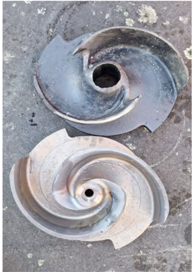
Figure 6: Pump no.1 damaged impellor replaced with new impellor and bolt.
