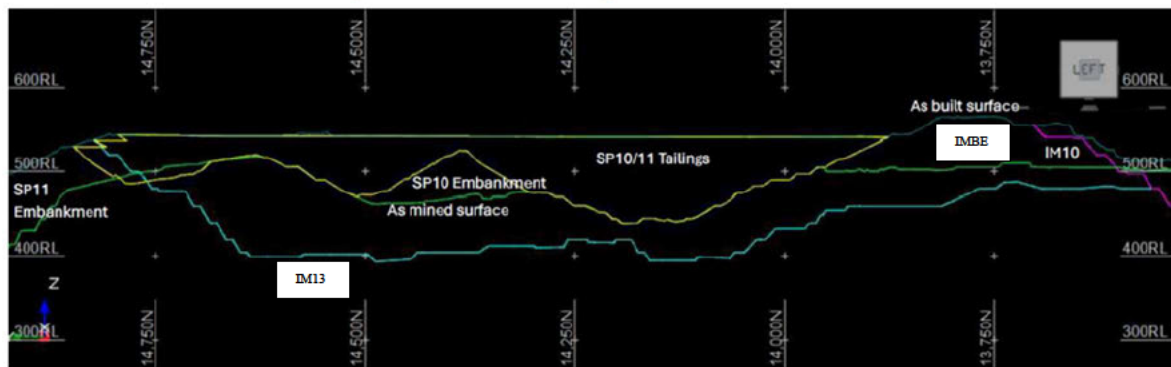
Figure 9: Section through 69,900 mE at SP11A, SP10 and IMBE
