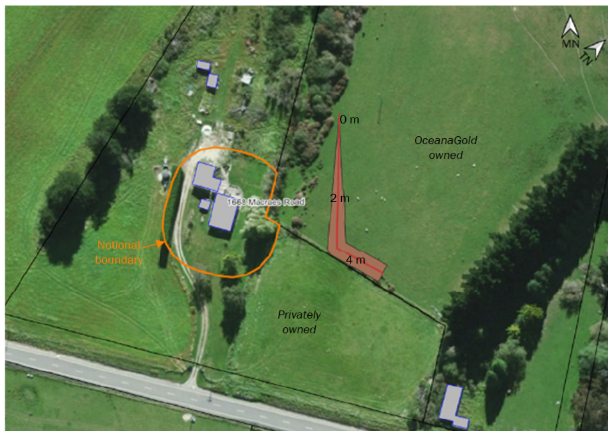
Figure 7.1 – Potential location for noise protection bund wall
