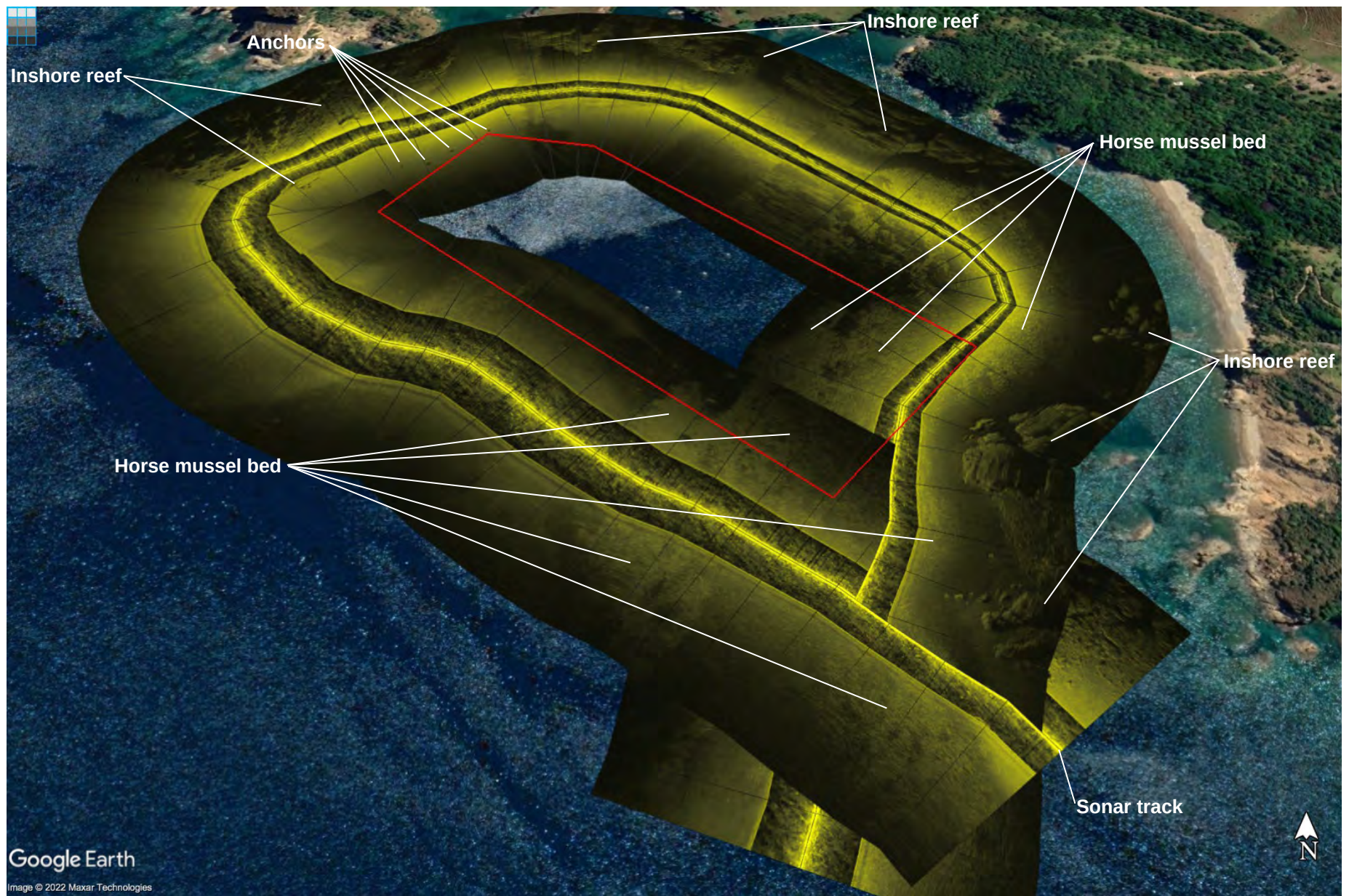
Figure 3.2. Example of the different habitats in the surveyed area and encountered via sonar during the field survey of the proposed 8009 AMA (as bounded in red). Note: representative drop camera imagery and live HD video feed were used to corroborate habitat types captured in side-scan sonar imagery.
