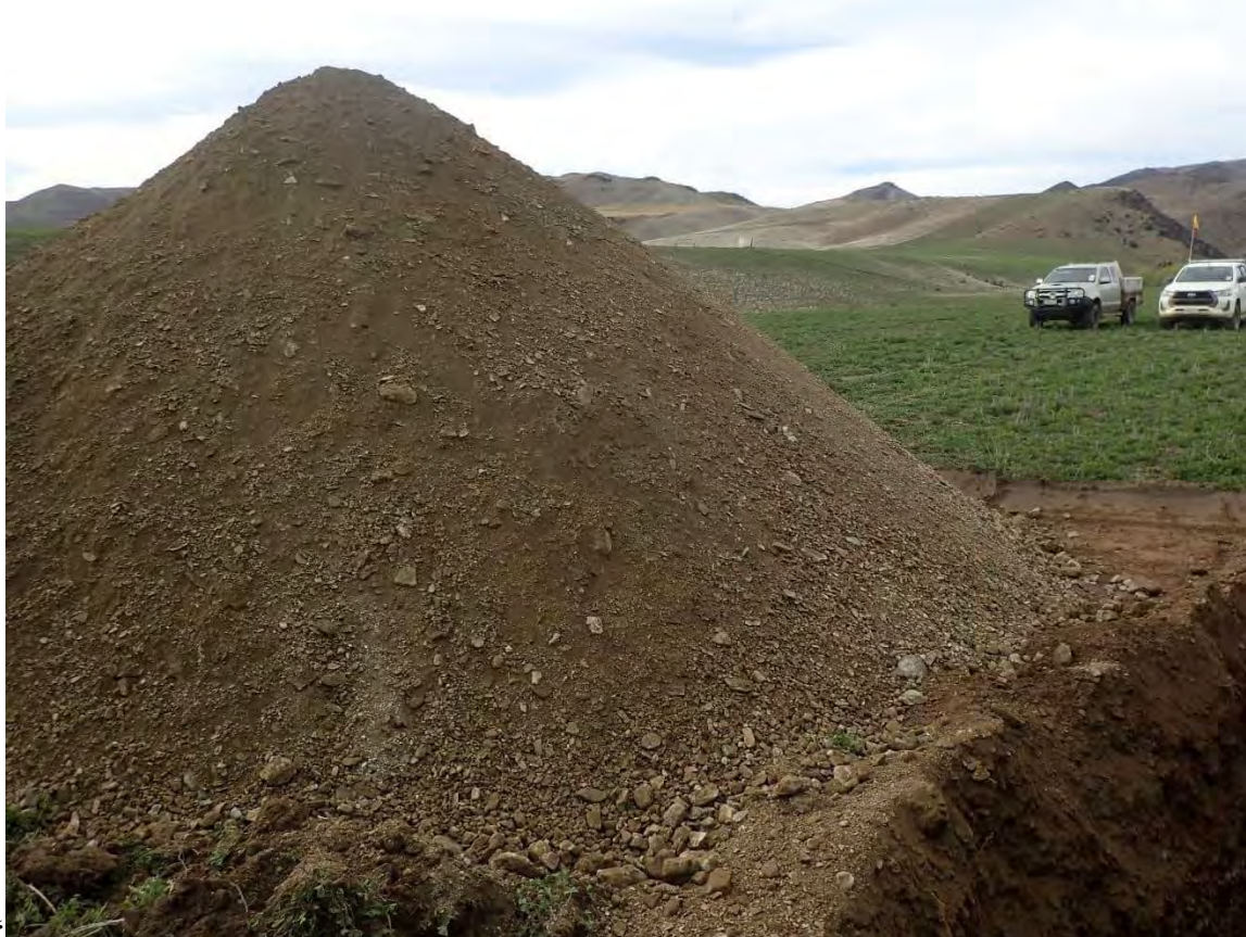
Testpit at completion. Max depth 6m
