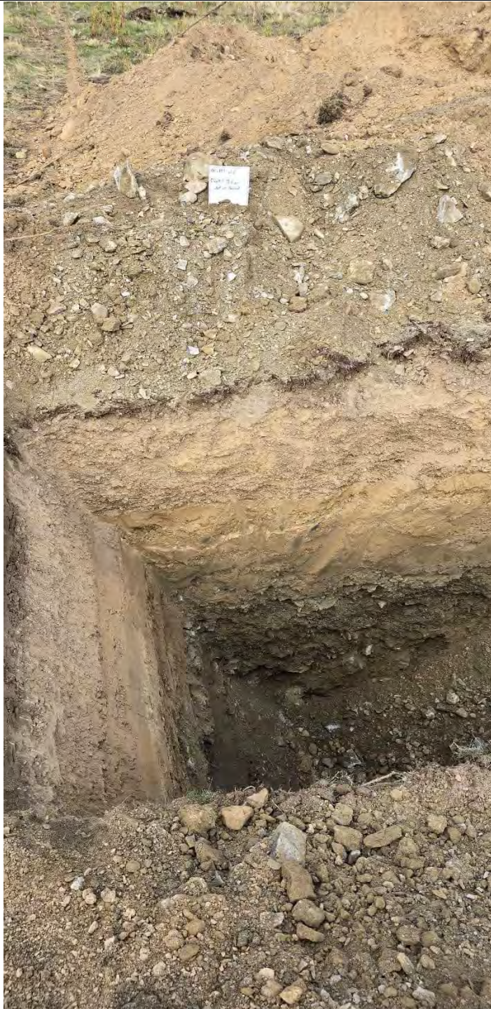
Testpit at completion. Max depth 3.1m
