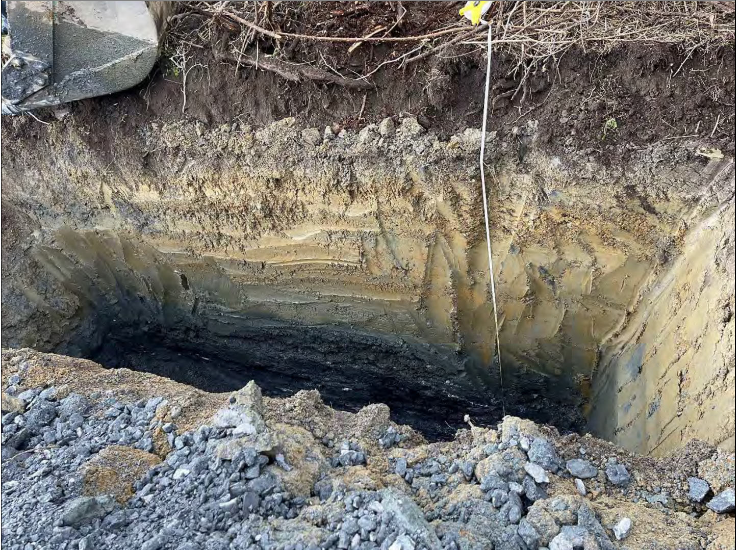
Testpit at completion. Max depth 3m
