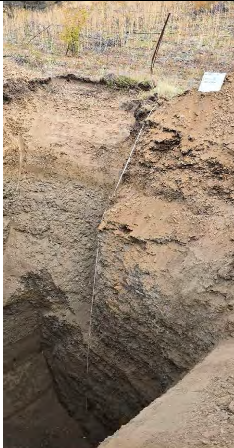
Testpit at completion. Max depth 6.9m
