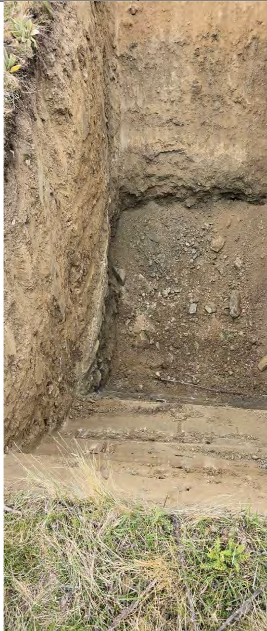
Testpit at completion. Max depth 3.5m
