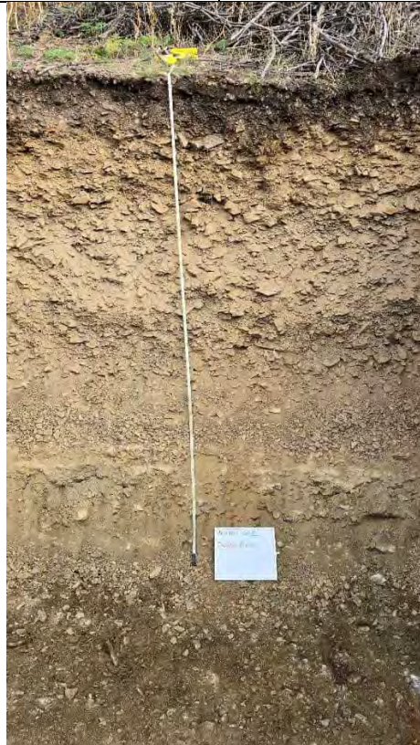
Testpit at completion. Max depth 2.8m
