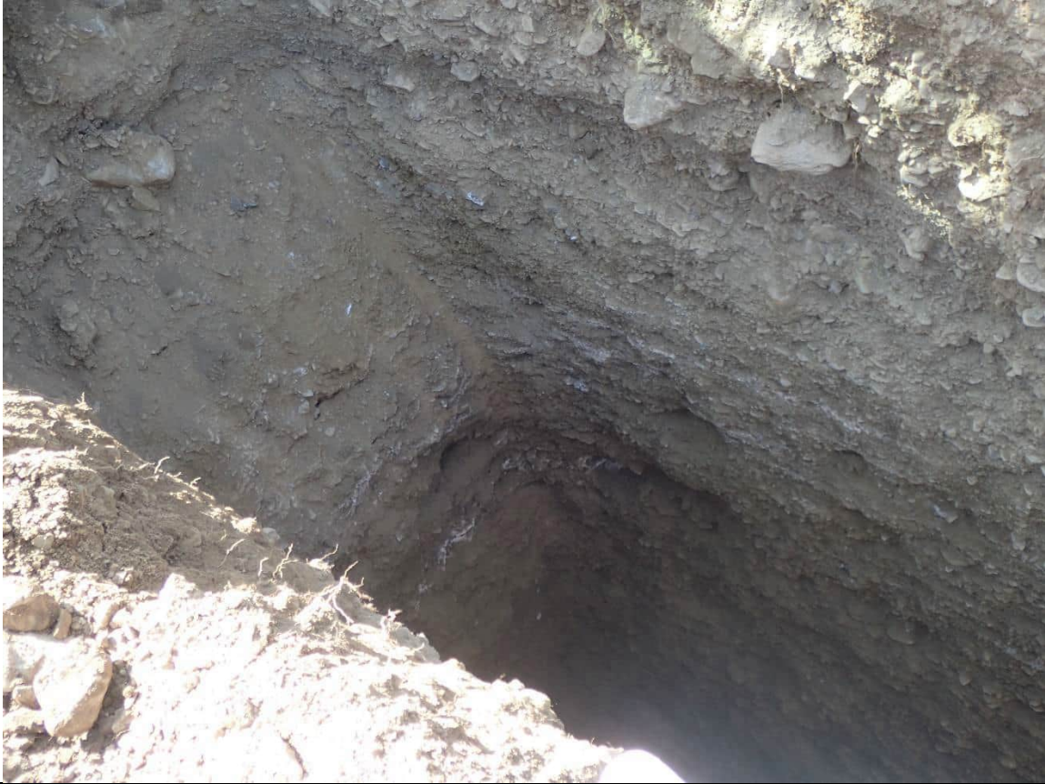
Testpit at completion. Max depth 7m
