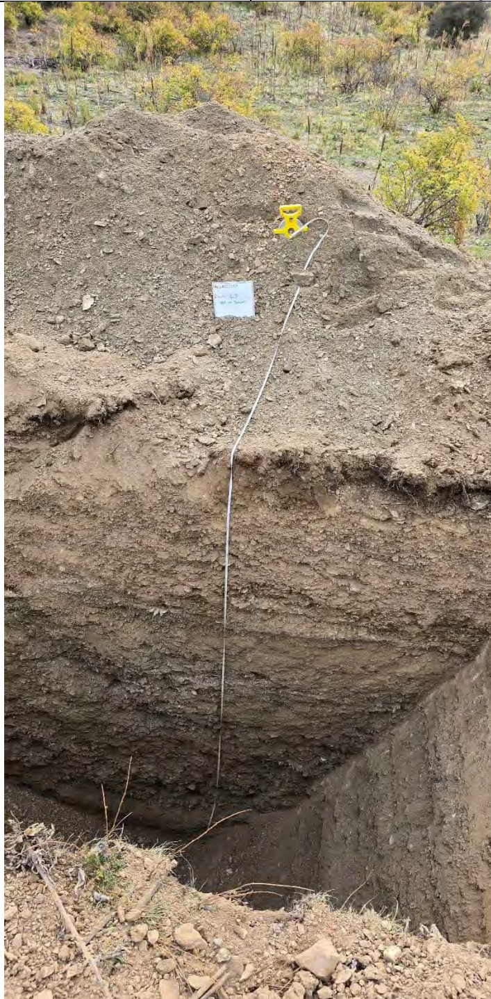
Testpit at completion. Max depth 4.12m
