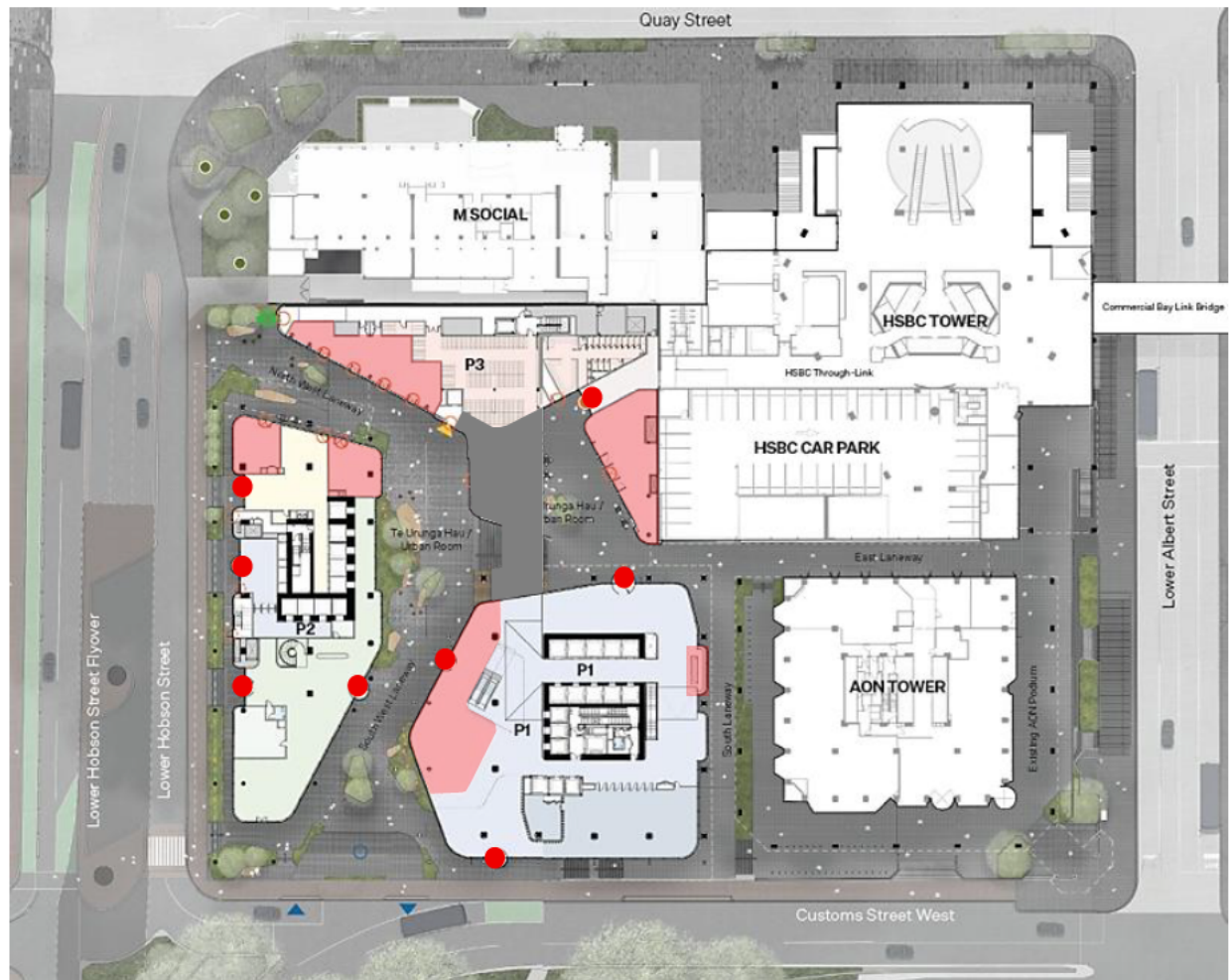
Figure 4.30 Hybrid plan showing lower ground floor under T2 at left (Level 00) and upper ground floor (Level 01) with entries (red circles) and indicative retail tenancies (pink).
