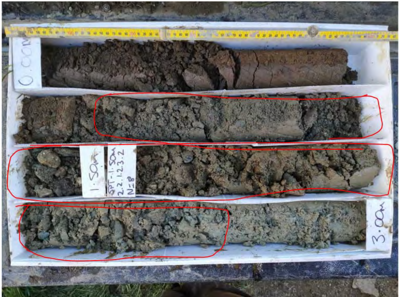
Figure 3, potentially liquefiable materials in BH_TT229892
