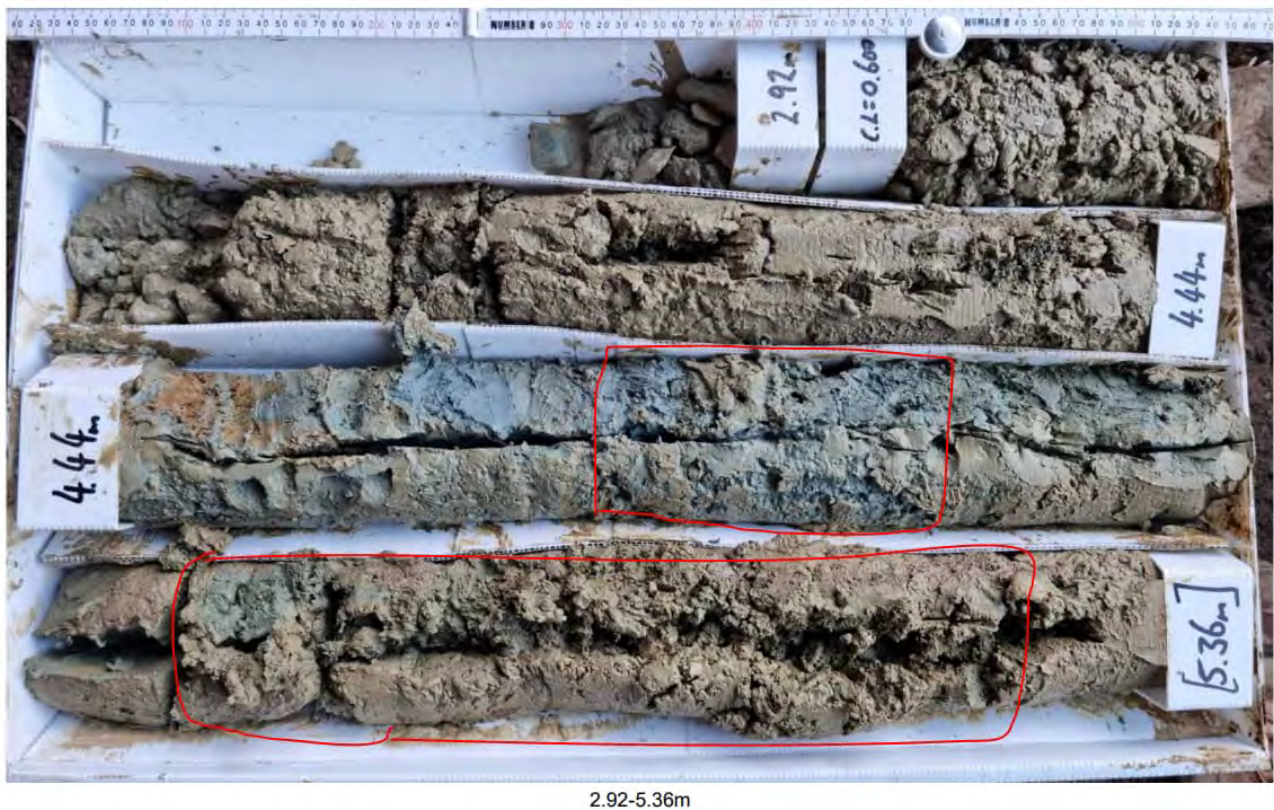
Figure 4, silty materials in BH_TT229896 that appear to have lower plasticity and are likely to be susceptible to liquefaction
