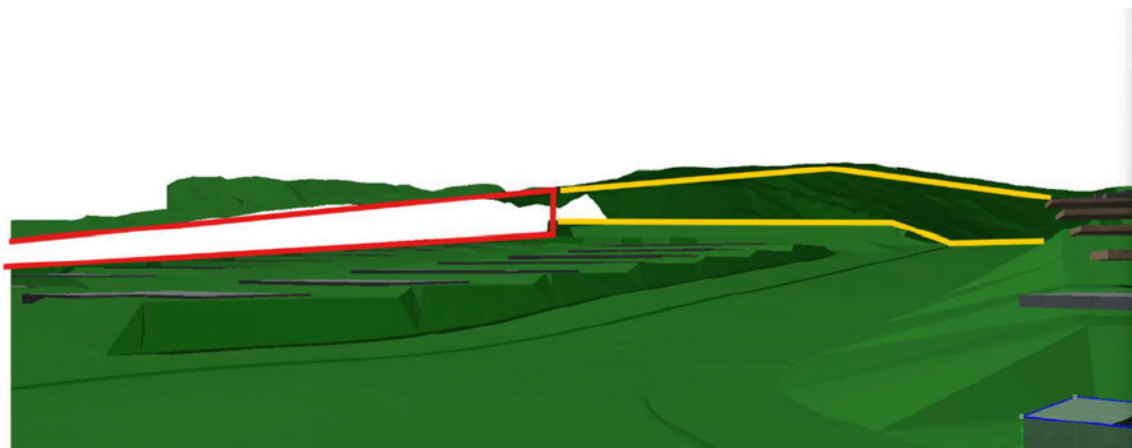
Figure 3 - Retaining walls required along the northern and eastern Delmore site boundaries to achieve compliant gradients along the NOR 6 arterial road.
