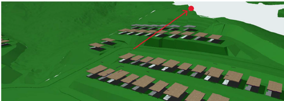
Figure 8 - Cross section highlighting the level differences between the Delmore Roding network and the paper road site boundary. A natural ground slope of approximately 1:4.5 or 22% prevents a road connection to the paper road at this location.
