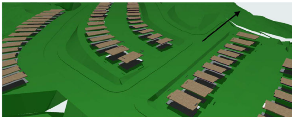
Figure 7 - 3D image highlighting the alignment of levels between Road 7 and the site boundary
