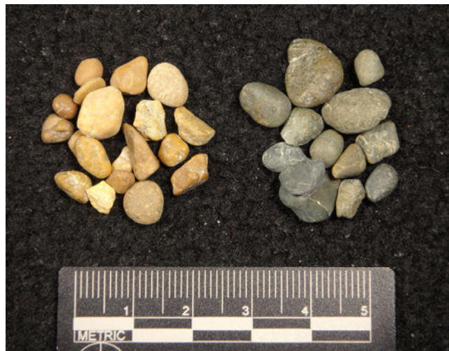
Image 2: Selection of pebbles and granules from coarse fraction of Ponar grab samples of Bream Bay sand. Pale particles at left are felsic volcanics. Grey particles at right are greywacke. All particles are in surface-dry state. Scale is in millimetres and centimetres.
