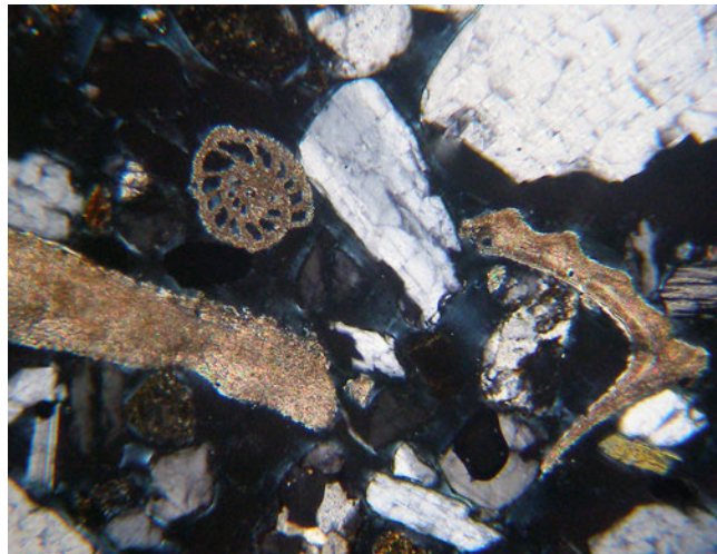
Image 10: Photomicrograph of Bream Bay sand, showing a single foraminiferan (upper left) and coarse molluscan fragments (pale brown and elongate). Quartz and feldspar show first order grey interference colours. Grains are set in isotropic mountant medium (dark). Same field of view as above, crossed polarisers, width of view 2.6 millimetres.
