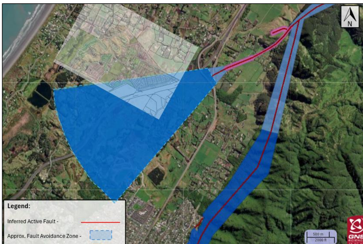
Figure 4. Overlay of the mapped Ōhāriu Fault and Fault Avoidance Zone (FAZ) on the Waikanae North Illustrative Masterplan (Landlink Ltd October 2025).
