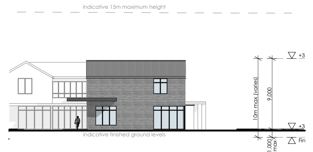
Workspace and Retail Two - South Elevation
