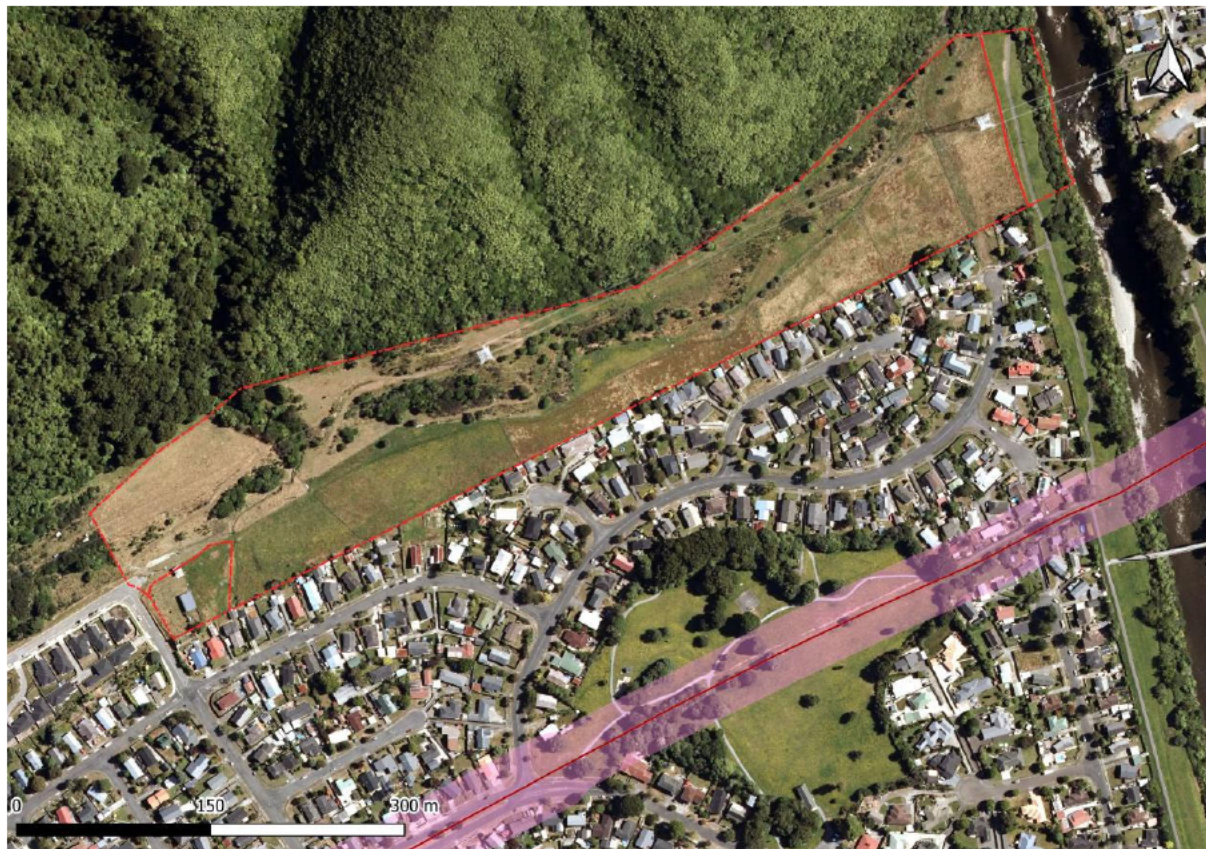
Figure 3: Wellington Fault Location and Confidence of Fault Location
