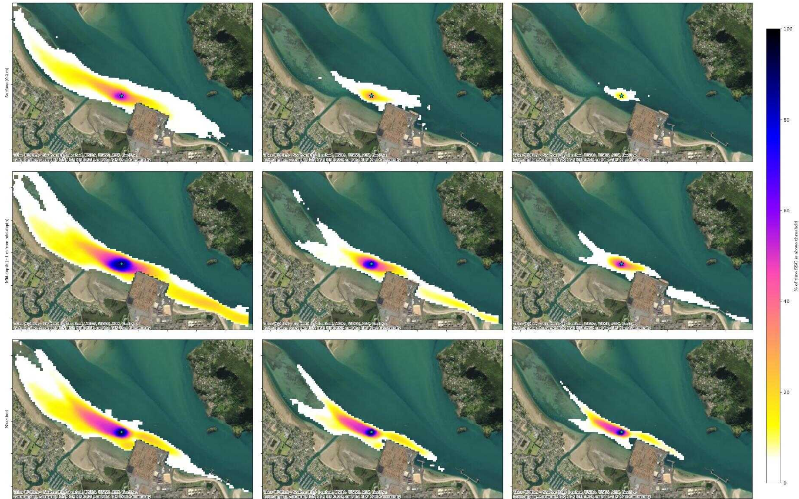
Figure 2 Percentage of time total suspended sediment concentrations ( \text{mg L}^{-1} ) are above thresholds of 2, 5, and 10 \text{mg L}^{-1} (left to right), at surface, mid water and nearbed levels (top to bottom) for BHD dredging at site 1 , over the existing bathymetry . Results are shown for the silty sand . Results were masked below 1%.
