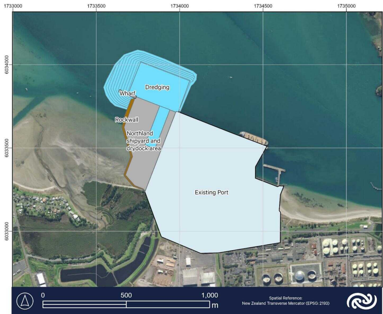
Figure 1-1 Concept drawing for the proposed area to be dredged and reclaimed for Design West.
