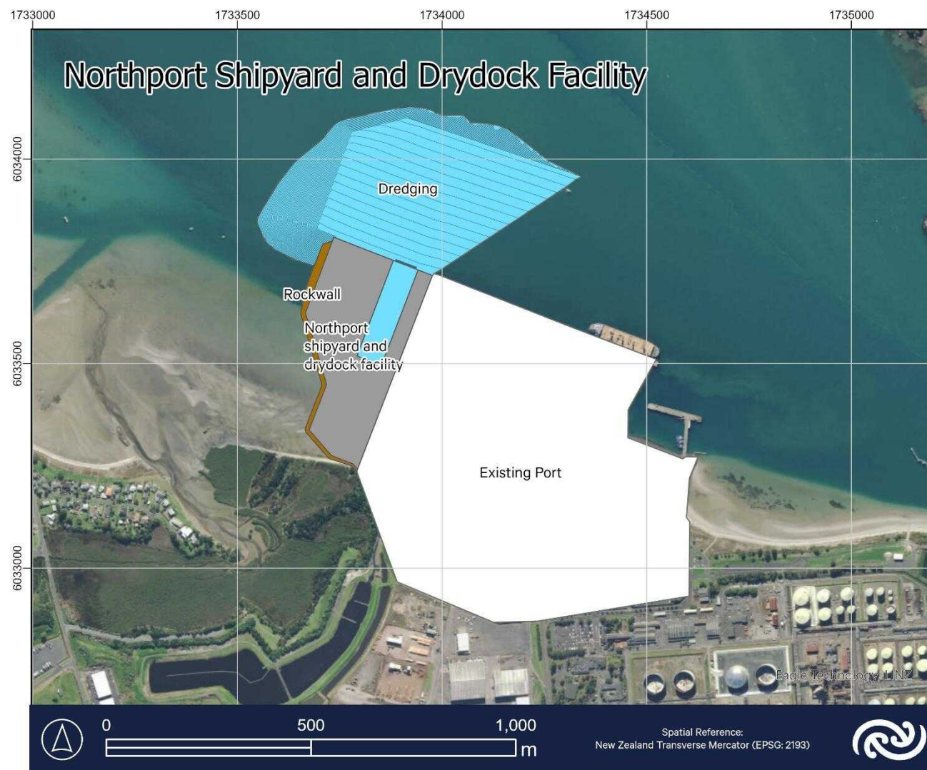
Figure 1-2 Concept drawing for the July 2026 design proposed area to be dredged and reclaimed for Design West.
