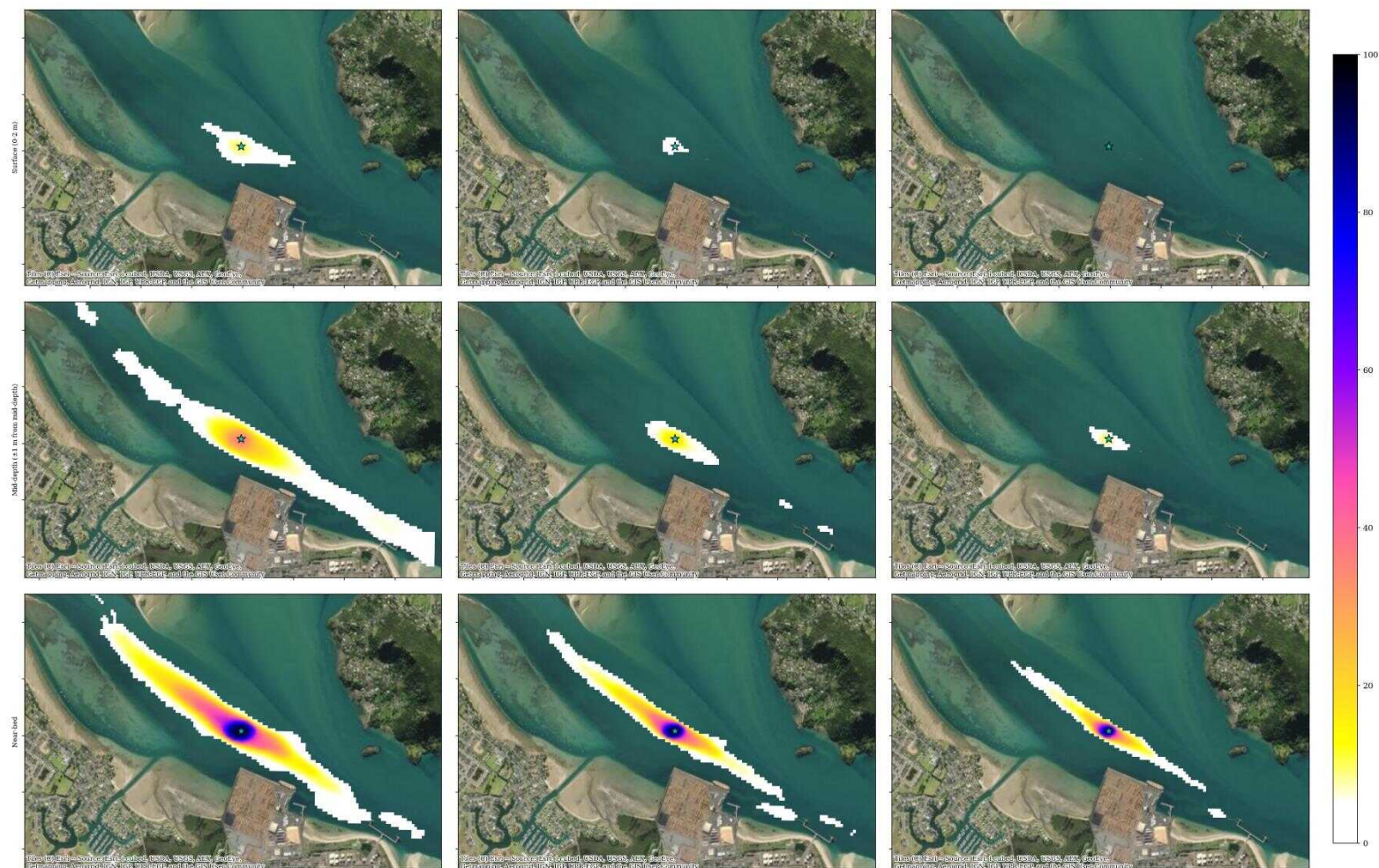
Figure 24 Percentage of time total suspended sediment concentrations (mg L -1 ) are above thresholds of 2, 5, and 10 mg L -1 (left to right), at surface, mid water and nearbed levels (top to bottom) for BHD dredging at site 4 , over the proposed NSDF bathymetry . Results are shown for the silty sand . Results were masked below 1%.
