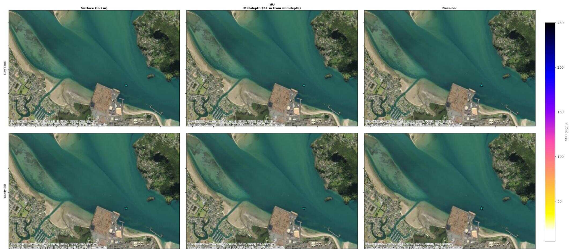
Figure 69 50th percentile of total suspended sediment concentrations ( \text{mg L}^{-1} ) at surface, mid water and nearbed levels (from left to right) for TSHD dredging at site 6 , over the existing bathymetry . Results are shown for the silty sand on the top panels and sandy silt on the bottom panel. The dredger is assumed to dredge continuously over the 1-month simulation period. TSS were masked below 5 \text{ mg L}^{-1} .
