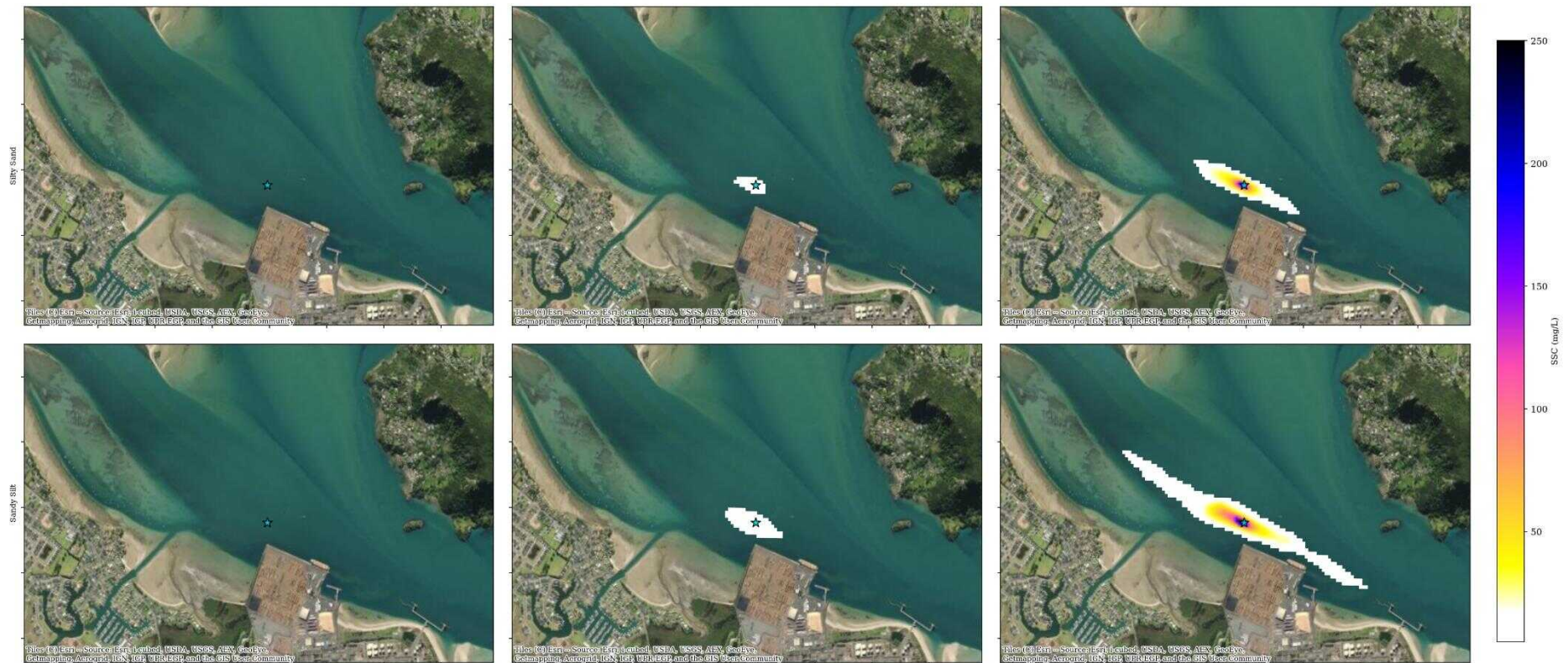
Figure 18 90 th percentile of total suspended sediment concentrations (mg L -1 ) at surface, mid water and nearbed levels (from left to right) for BHD dredging at site 3 , over the proposed NSDF bathymetry . Results are shown for the silty sand on the top panels and sandy silt on the bottom panel. The dredger is assumed to dredge continuously over the 1-month simulation period. TSS were masked below 5 mg L -1
