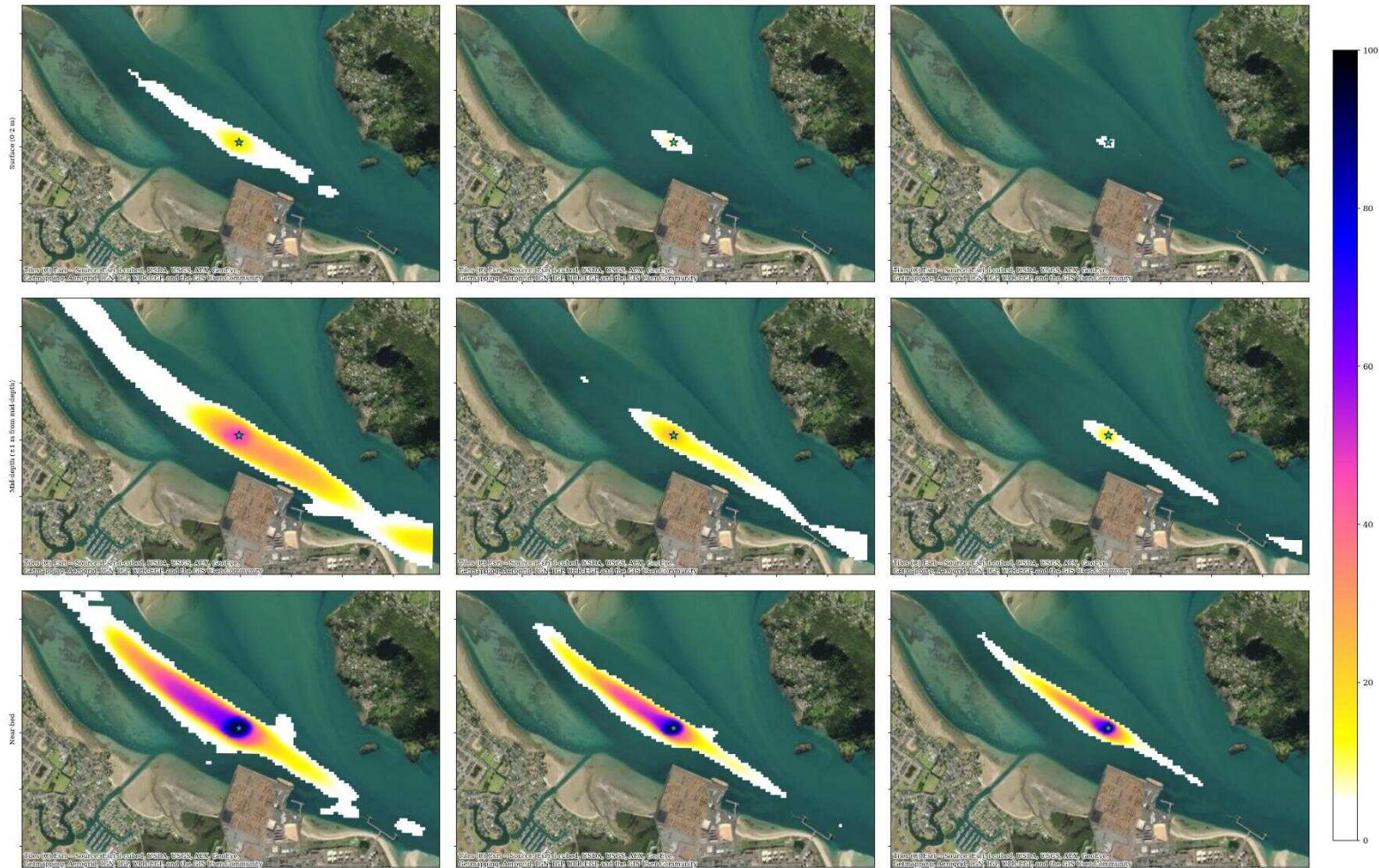
Figure 20 Percentage of time total suspended sediment concentrations (mg L -1 ) are above thresholds of 2, 5, and 10 mg L -1 (left to right), at surface, mid water and nearbed levels (top to bottom) for BHD dredging at site 4 , over the existing bathymetry . Results are shown for the silty sand . Results were masked below 1%.
